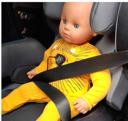
FIGURE 22. Photography of baby emulator in a seat with an electromechanical transducer.
