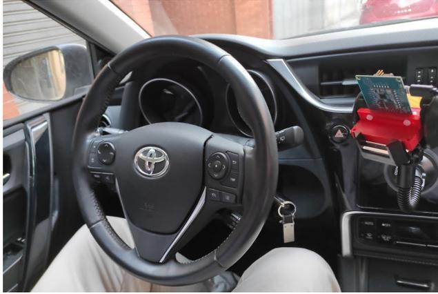
FIGURE 5. Image of the radar installer in the car oriented to the driver.
