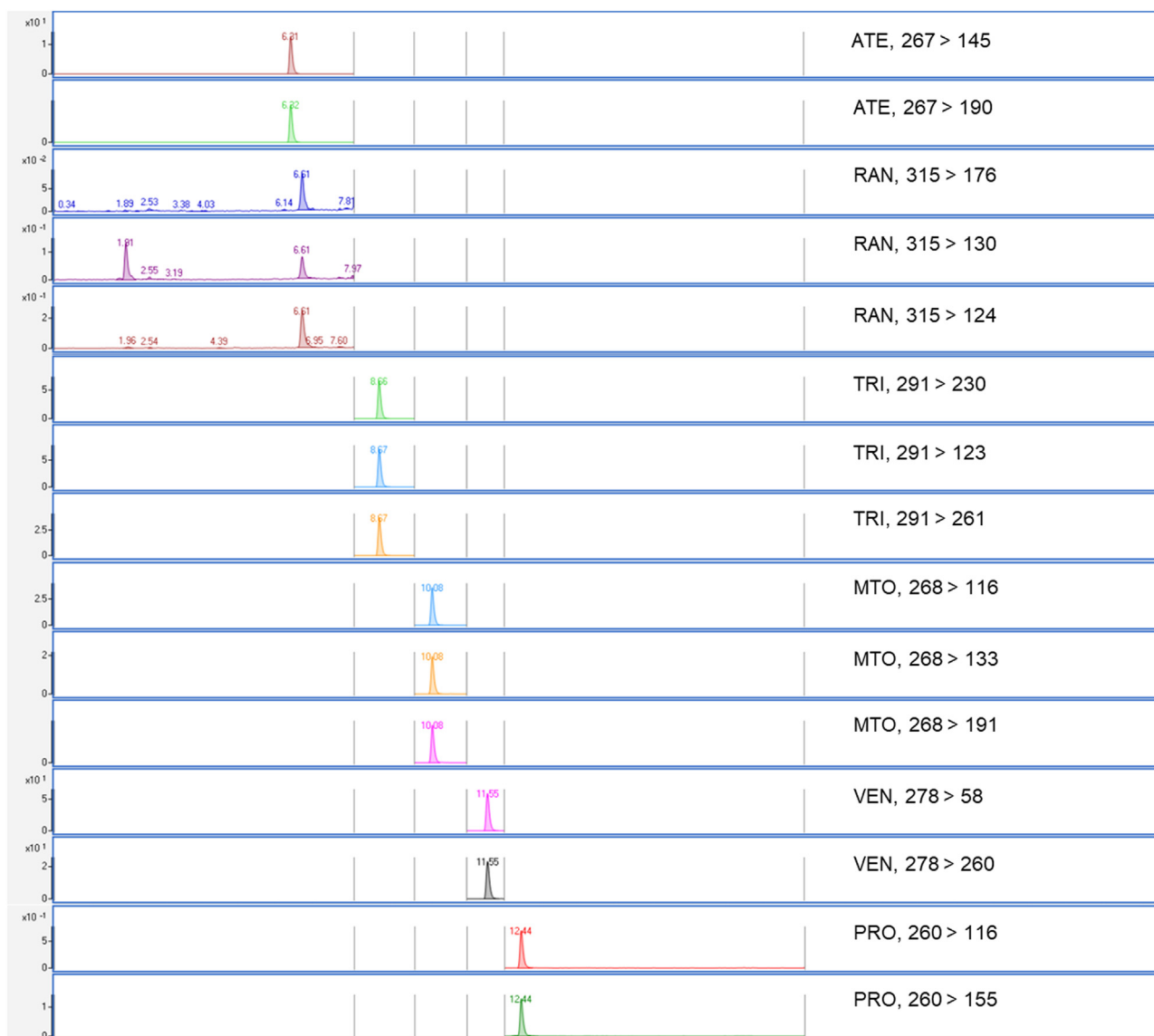
Fig. 5. Chromatogram of an effluent wastewater sample when it was analyzed using the developed method.
