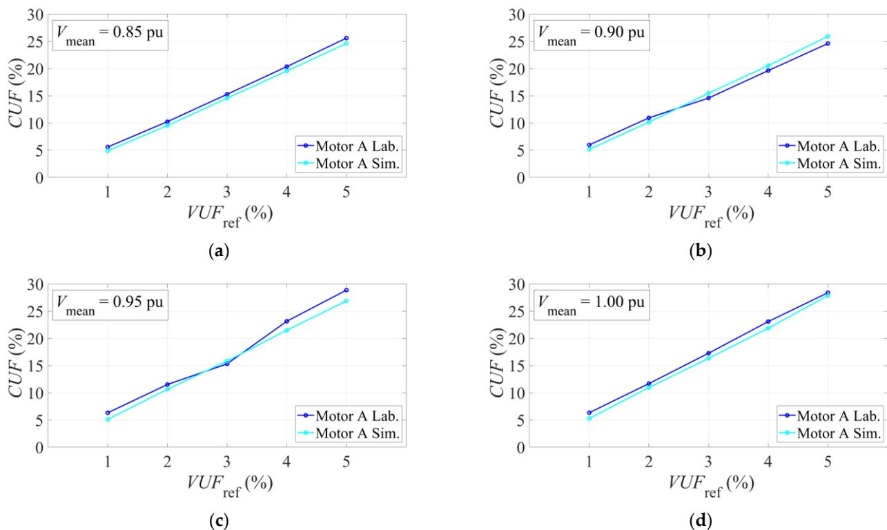
**Figure 4.** CUF vs. VUF on motor A for experimental (blue) and simulation (cyan) results, and different values of  $V_{\text{mean}}$ : (a) 0.85 pu; (b) 0.90 pu; (c) 0.95 pu; (d) 1.00 pu.
