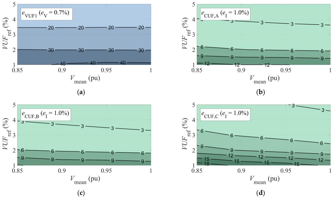
**Figure 5.** (a)  $VUF$  error ( $e_{VUF_1}$ ) according to  $V_{mean}$  and  $VUF_{ref}$  when the measurement error in the voltmeters is 0.7%;  $CUF$  error ( $e_{CUF}$ ) according to  $V_{mean}$  and  $VUF_{ref}$  when the measurement error in the ammeters is 1.0%: (b) Motor A; (c) Motor B; (d) Motor C.
