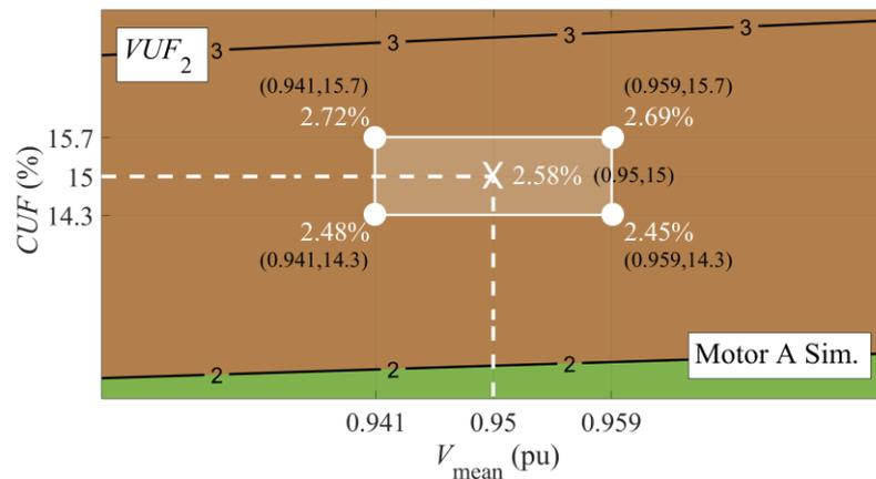
Figure 7.  $VUF_2$  according to measurement errors.
