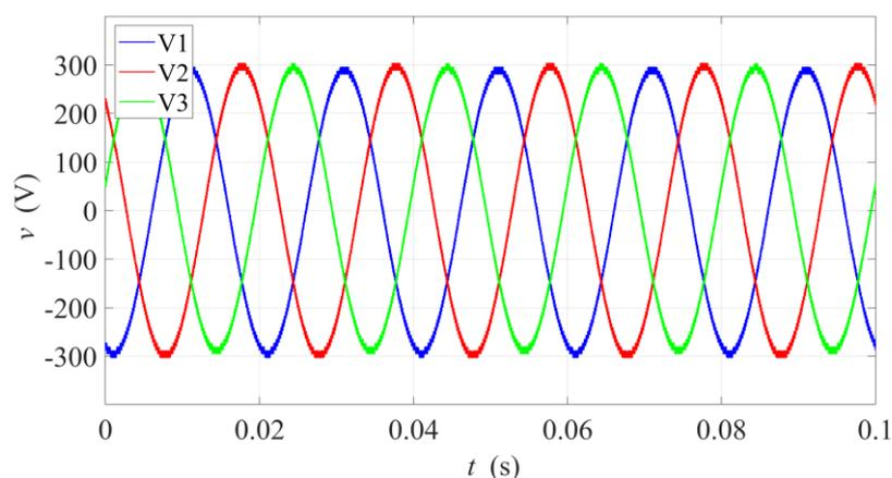
**Figure 1.** Three-line unbalance voltages for Point 2 in Table 1, with  $VUF_{ref} = 1\%$  and  $V_{mean,ref} = 0.90$ .
