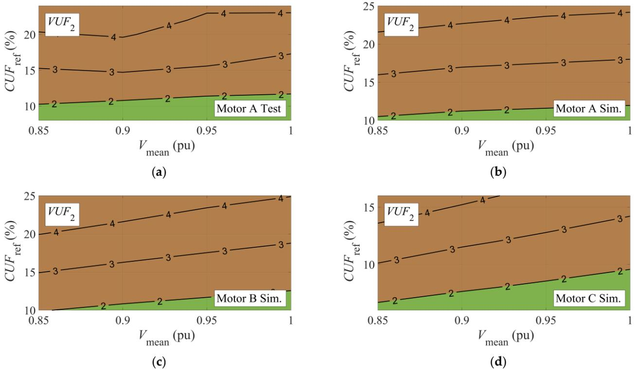
Figure 6.  $VUF_2$  according to  $V_{mean}$  and  $CUF$  for: (a) Test results for Motor A; (b) Simulation results for Motor A; (c) Simulation results for Motor B; (d) Simulation results for Motor C.
