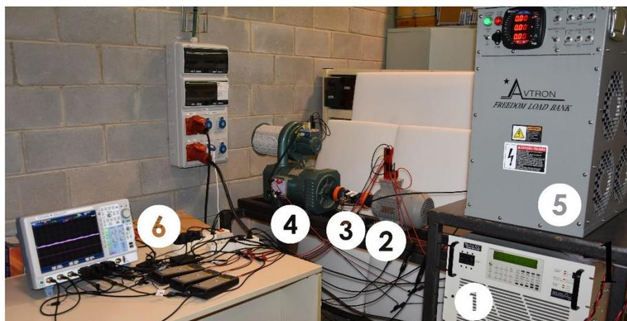
**Figure 3.** General overview of laboratory setup used in the tests. The main devices are: (1) programmable power source; (2) induction motor; (3) torque and speed sensors; (4) DC generator; (5) DC generator's resistive load; (6) oscilloscope.
