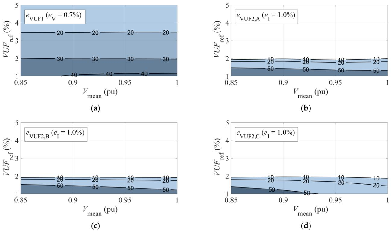
**Figure 8.** *VUF* error according to *VUF* and  $V_{\text{mean}}$ : (a) for Motor A, obtained from  $e_{VUF1}$ ; (b) for Motor A, obtained from  $e_{VUF2,A}$ ; (c) for Motor B, obtained from  $e_{VUF2,B}$ ; (d) for Motor C, obtained from  $e_{VUF2,C}$ .
