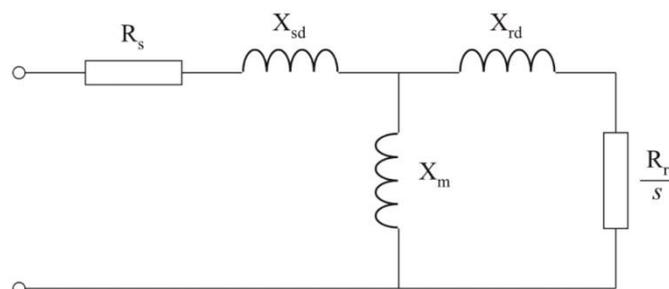
**Figure 2.** Equivalent circuit with five constant parameters for the single-cage model of the induction motor.
