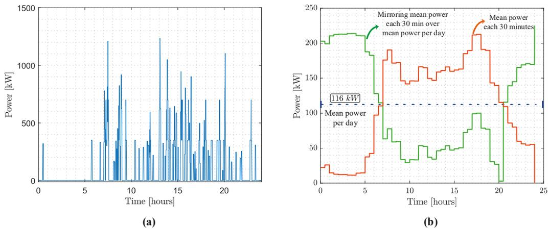
Fig. 4. (a) Demanded daily power profile of 100 EVs predicted by Montecarlo simulation; (b) Average consume profile for 1000 days predicted by Montecarlo simulation.
