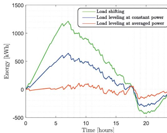
Figure 5. ESS charging /discharging dynamics during one operating day for different energy management strategies.
