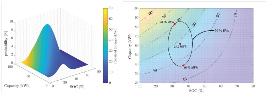
Fig. 3. Required energy to attain 80 % SOC in the EV battery.
