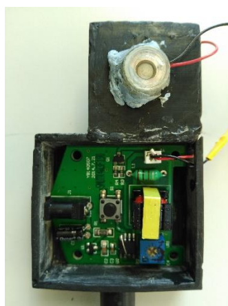
Figure 5: Acoustic Wave Nebulizer (AWN)
