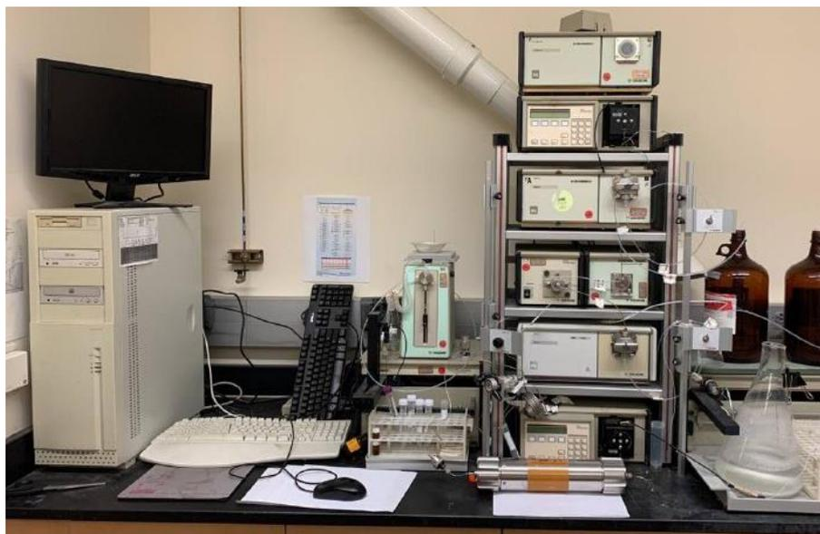
**Figure 14.** Set up for the preparative HPLC.
