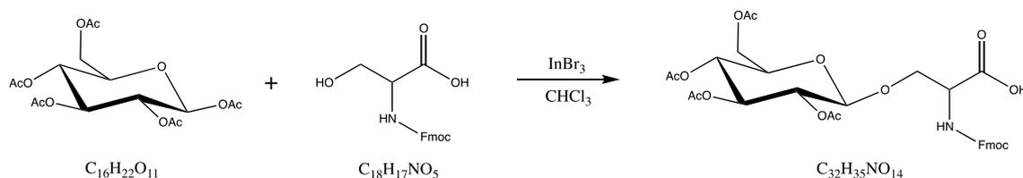
**Figure 9.** Reaction scheme for the glycosylation of N-Fmoc-Serine-OH with  $\beta$ -Peracetyl Glucose.
