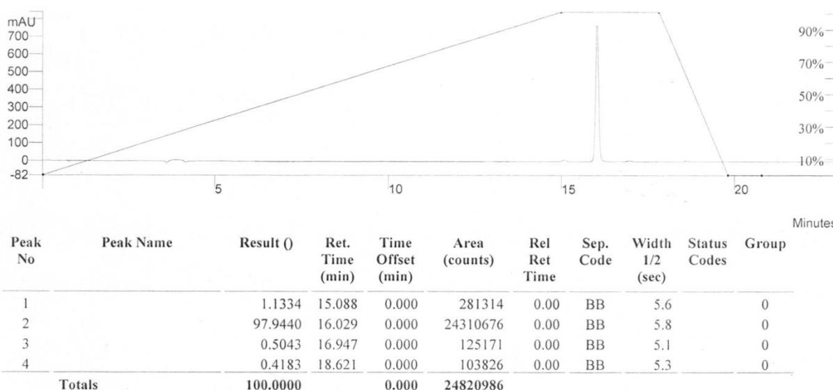
**Figure 15.** HPLC of the first batch of Fmoc-Ser(Glc(OAc)<sub>4</sub>)-OH.
