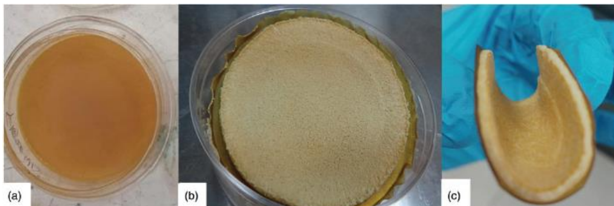
Figure 9 Soy protein-based wound dressings: (a) dense monolayer film; (b) hybrid film; (c) a hybrid film being bent to demonstrate its flexibility. Adapted from (Matsliah et al., 2021)
