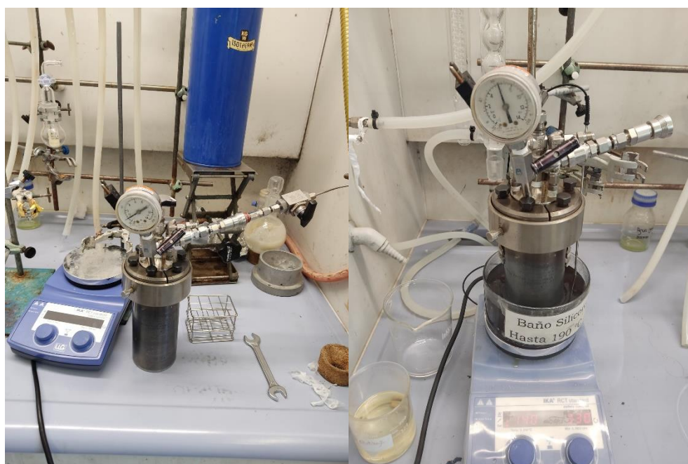
Figure 8. Experimental set-up for the synthesis of styrene carbonate
