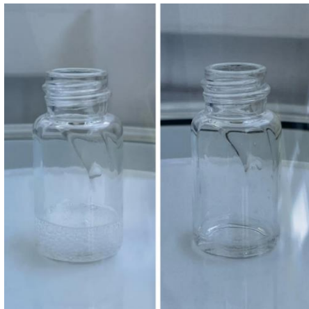
Figure 15. Before and after of degasification of PDMS
