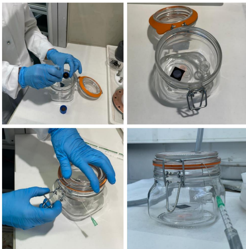
Figure 13. FOTS steps to modify PSi surface
