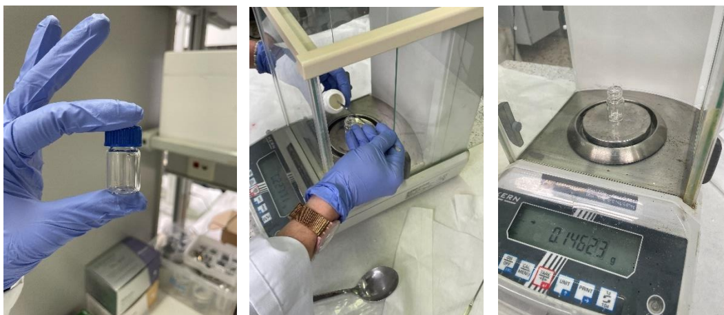
Figure 17. Preparing PGLA; (1) Tiny container where we are going to prepare our mixture; (2) and (3) measuring quantity of PGLA needed
