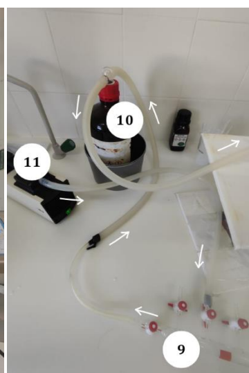
Figure 10 - Vacuum circuit. (9) Vacuum manifold (10) Pressure regulator (11) Diaphragm pump
