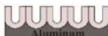
Figure 7. Schematics depicting the cross-section view of the pores after the 2nd anodization process.
