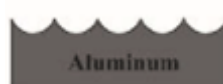
Figure 6. Schematics depicting the cross-section view of the nucleative centers formed after removal of unordered pores.
