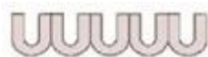
Figure 8. Schematics depicting the cross-section view of the pores after aluminium layer removal.
