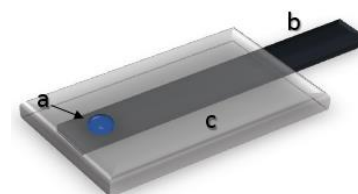
Figure 2.1. Scheme of the potentiometric paper based sensor: a) circular window with drop-casted Nafion membrane; b) free area of platinumized paper used as the electric contact; c) plastic mask.
