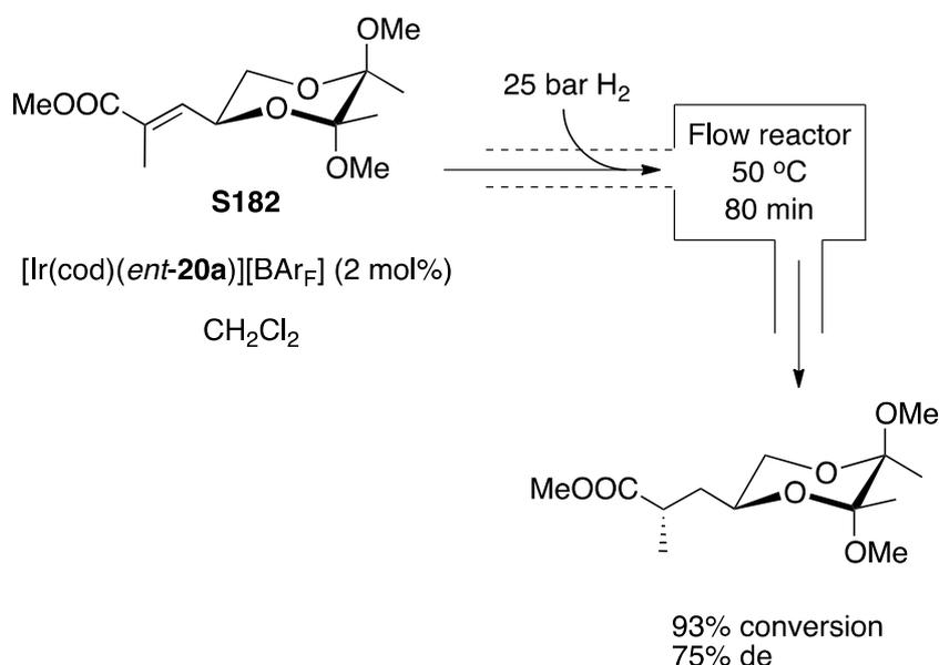
**Scheme 31** Diastereoselective hydrogenation of **S182** performed in a flow reactor setup.
