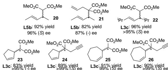
**Figure 2.** Pd-allylic substitution of **S3-S6**. Full conversions were achieved. 0.5 mol % [PdCl(η<sup>3</sup>-C<sub>3</sub>H<sub>5</sub>)<sub>2</sub>], CH<sub>2</sub>Cl<sub>2</sub> as solvent, ligand (1 mol %), rt, 18 h.
