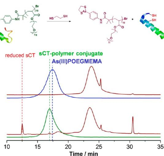
**Figure 11.** (a) Conjugation of sCT to As(III)POEGMEMA (2.5 equiv) via sequential reduction conjugation. (b) Release of sCT from the sCT-POEGMEMA conjugate using 1,2-ethanedithiol (bottom spectra) and control reaction of 4 and EDT (top spectra). Adapted with permission from ref 229. Copyright 2015 American Chemical Society.
