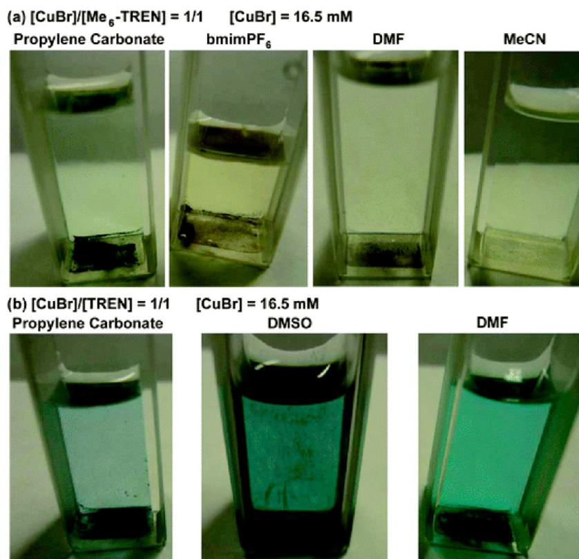
**Figure 2.** Visual observation of Cu(0) nanoparticles and CuBr<sub>2</sub> generated from the disproportionation of CuBr in polar aprotic solvents in the presence of Me<sub>6</sub>-TREN (a) and TREN (b). Conditions: solvent = 1.8 mL; [CuBr]/[N-ligand] = 1:1. Pictures were taken 10 min after mixing the reagents. Reproduced from ref 14, with permission of The Royal Society of Chemistry. <http://dx.doi.org/10.1039/C2PY21084C>.
