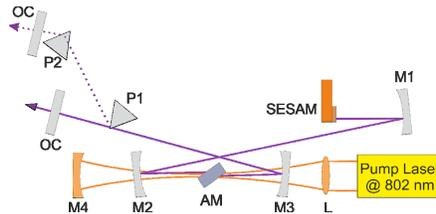
Fig. 1. Layout of the  $\text{Tm,Ho:KLuW}$  laser. AM: active medium; L: focusing lens; M1: concave mirror (radius of curvature  $\text{RoC} = 50 \text{ mm}$ ); M2, M3 and M4: concave mirrors ( $\text{RoC} = 100 \text{ mm}$ ); M1, M2, M3: highly reflective at 2060 nm and highly transmitting at 800 nm; M4: highly reflective at 800 nm; P1 and P2:  $\text{CaF}_2$ -prisms; OC: output coupler.
