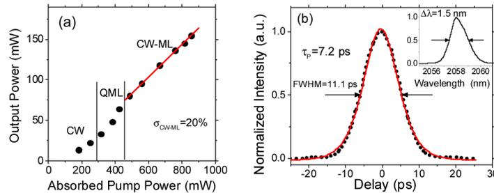
Fig. 2. SESAM mode-locked Tm,Ho:KLuW laser ( $T_{oc} = 3\%$ , SESAM No.2): (a) output vs. input characteristics (dots) and linear fit in the mode-locked (CW-ML) regime (red line); (b) autocorrelation curve (black dots), fit assuming  $\text{sech}^2$  pulse shape (red line) and optical spectrum (inset).
