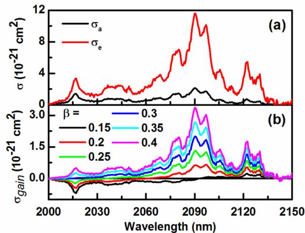
Fig. 1. Spectroscopic characterization of the 1% Ho-doped YAG ceramics in the 2- $\mu\text{m}$  region. (a) Absorption  $\sigma_a$  and emission  $\sigma_e$  cross section. (b) Gain cross section  $\sigma_{gain}$  for different inversion levels  $\beta$ .
