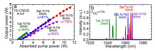
Fig. 6. Comparison of the laser performance of *a*-cut Yb:CNGS crystals with various Yb<sup>3+</sup> doping levels ( $T_{OC} = 1\%$ ,  $\sigma$ -polarization): (a) input-output dependences,  $\eta$  – slope efficiency; (b) typical laser emission spectra measured at maximum  $P_{abs}$ .
