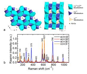
Fig. 2. Structural study of a 5 at.% Yb:CNGS crystal: (a) fragment of the CNGS structure in projection to the *a-b* and *b-c* planes; (b) polarized Raman spectra,  $\lambda_{exc} = 514$  nm.
