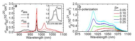
Fig. 3. Spectroscopy of the trigonal Yb:CNGS crystal: (a) absorption,  $\sigma_{abs}$ , and stimulatedemission,  $\sigma_{SE}$ , cross-sections for  $\pi$  and  $\sigma$ -polarizations, *inset* – the spectrum around the ZPL; (b) gain cross-sections,  $\sigma_g = \beta \sigma_{SE} - (1 - \beta)\sigma_{abs}$ , for  $\sigma$ -polarization,  $\beta$  is the inversion ratio,  $\beta = N_2/N_{Yb}$ .
