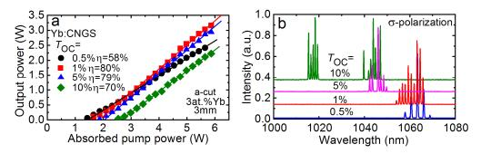
Fig. 5. Continuous-wave Yb:CNGS laser: (a) input-output dependences,  $\eta$  – slope efficiency; (b) typical laser emission spectra measured at  $P_{abs} = 5.5$  W (*a*-cut crystal, 3 at.% Yb<sup>3+</sup>, 3 mm-thick).
