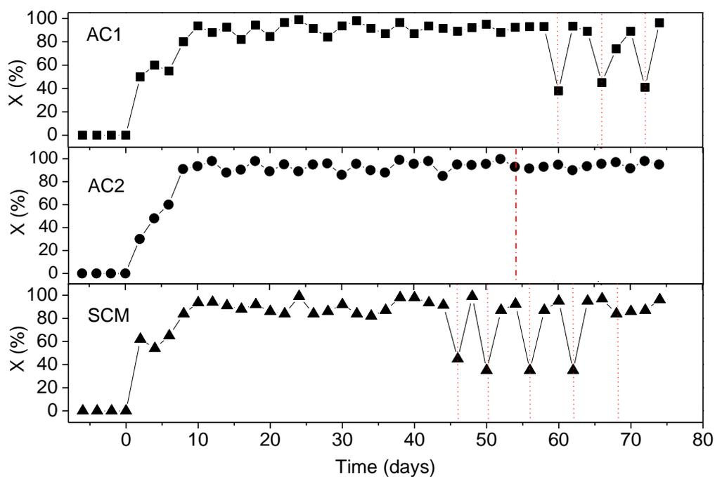
**Figure 3.** Effect of slow agitation in three up-flow stirred packed-bed reactors, two of which were filled with activated carbon as catalytic support material (USPBR-BAC1 and USPBR-BAC2) and the other with sludge carbonaceous material (USPBR-BSCM): nitrate removal (X); the dashed line shows the agitation applied on some days.
