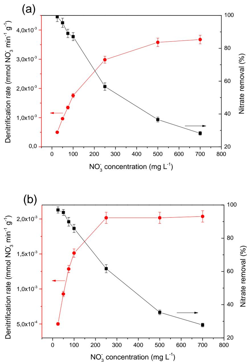
**Figure 4. Denitrification rate ( ) and nitrate removal ( ) versus nitrate concentration. (a) USPBR-BSCM, (b) USPBR-BAC.**
