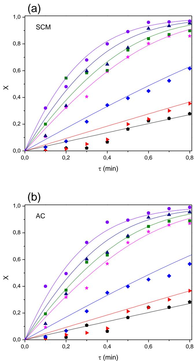
**Figure 5. Kinetic modelling of nitrate removal in (a) USPBR-BSCM, (b) USPBR-BAC. Nitrate concentrations: 25 mg·L<sup>-1</sup> (◆), 50 mg·L<sup>-1</sup> (▶), 75 mg·L<sup>-1</sup> (●), 100 mg·L<sup>-1</sup> (●), 250 mg·L<sup>-1</sup> (▲), 500 mg·L<sup>-1</sup> (■), 700 mg·L<sup>-1</sup> (★); lines represent the fit to the Michaelis-Menten model. X: nitrate removal rate (mmol·min<sup>-1</sup>·g<sup>-1</sup>), τ: space time (min).**
