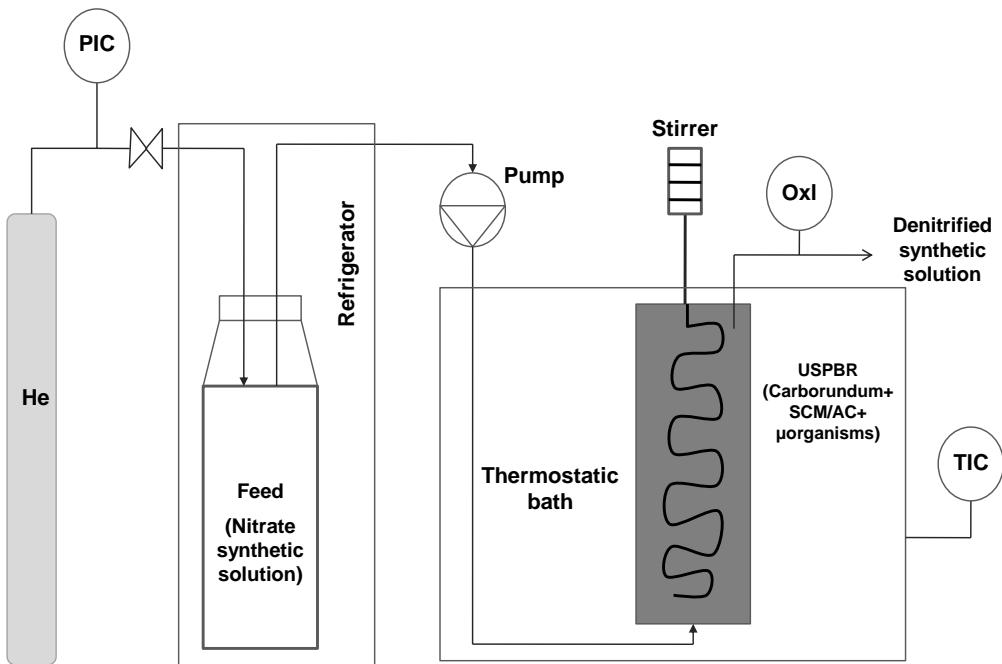
**Figure 1. Anaerobic USPBR system**
