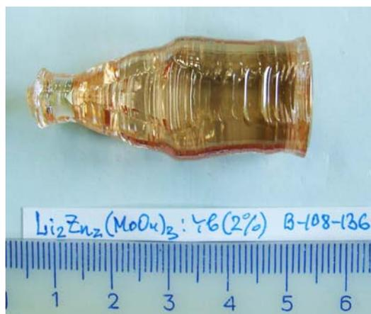
**Figure 1** Photograph of the as-grown boules of the LiZnMo crystal doped with (nominally) 2 at.% Yb; the growth direction is along the [010] axis.
