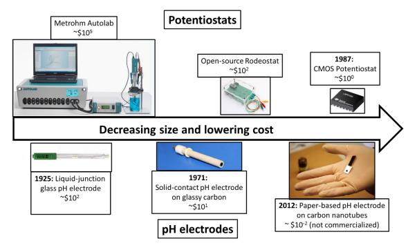
*Figure 2.* Decreasing size and cost of potentiostats (above) and pH electrodes (below).
