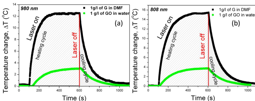
Figure 3. (a) Temperature profile of the G and GO under the same conditions with 980 nm irradiation wavelength; (b) Temperature profile of G and GO at 808 nm irradiation wavelength.
