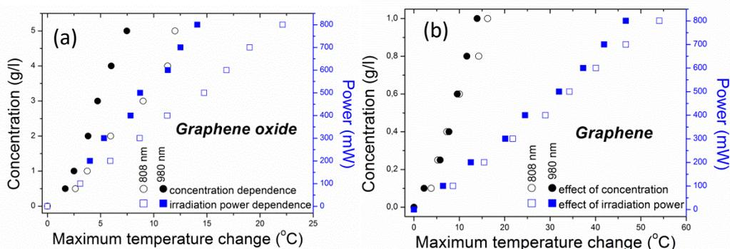
Figure 4. Temperature change under 980 and 808 nm laser irradiation at different concentrations and different irradiation powers of (a) GOnanosheets dispersed in water, and (b) G nanosheets dispersed in DMF.
