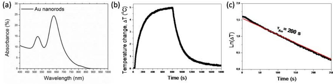
Figure 6. (a) Absorption spectrum of Au nanorods, 25 nm in diameter and 50 nm in length. (b) Temperature profile generated by Au nanorods being excited at 650 nm with a diode laser. (c) Time constant for heat transfer of the Au nanorods by applying the natural logarithm of temperature change versus time data, which is obtained from the cooling cycle shown in panel (b).
