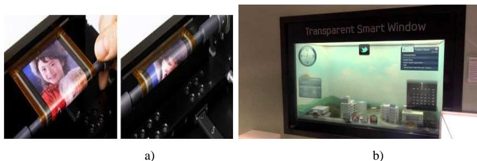
Fig. 1.5. a) SONY's organic thin film transistor driven, full color, flexible OLED display (80  $\mu\text{m}$ -thick and 4 inches wide), able to reproduce moving images while being rolled around a cylinder with a radius of 4 mm., b) SAMSUNG's transparent smart window.
