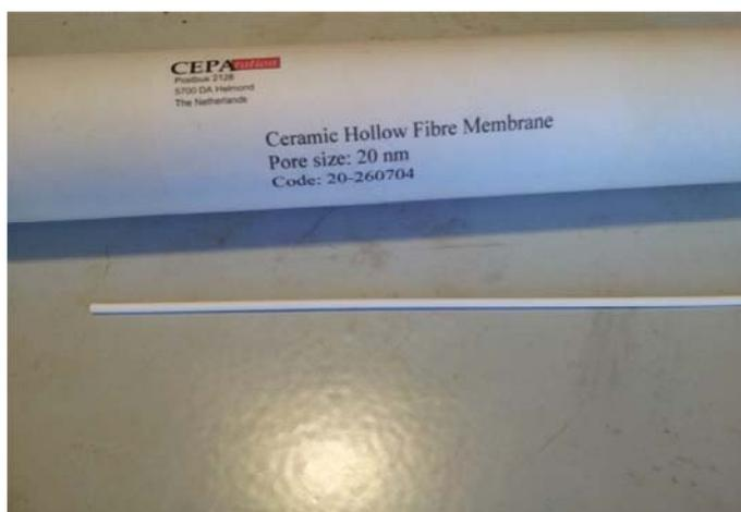
Figure 4-1 Single ceramic hollow fiber membrane
