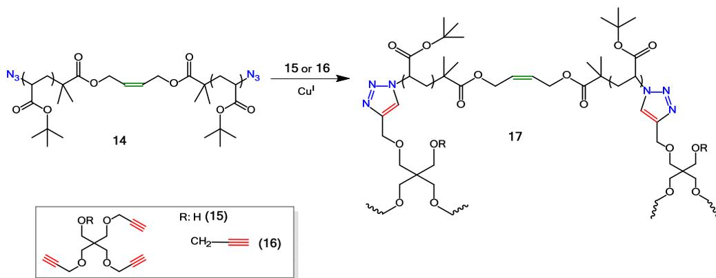
**Scheme 9.** Degradable polymer networks through CuAAC polymerization.
