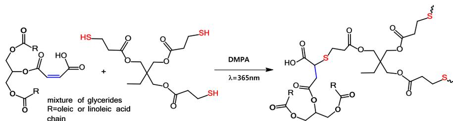
**Scheme 31.** Thiourethane thermoset coatings prepared by thiol-ene polymerization.
