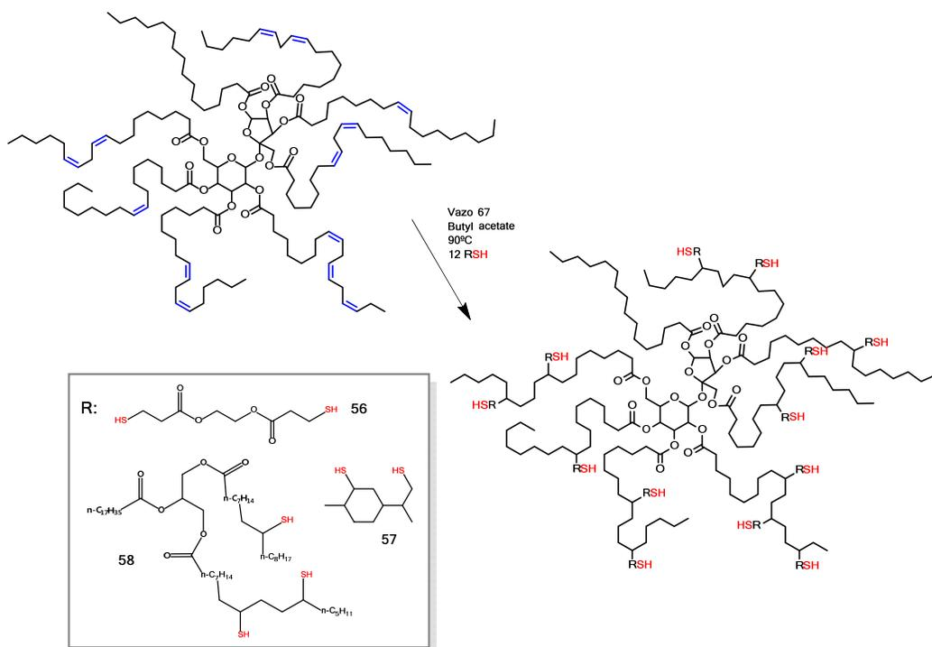
**Scheme 29.** Thiourethane thermoset coatings prepared by thiol-ene polymerization.
