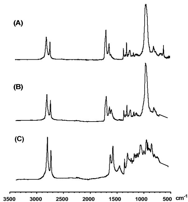
**Supporting Figure SF3.** FTIR spectra of PA-UDS degrading in phosphate buffer (pH 7.4) at 37°C. (A) Before degradation; (B) after degradation of 5 h; (C) after degradation of 60 h.
