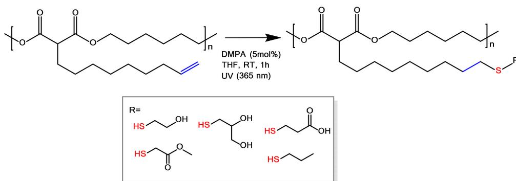
**Scheme 37.** Post-polymerization modification of the side chains of alkene-functionalized poly(malonate)s.
