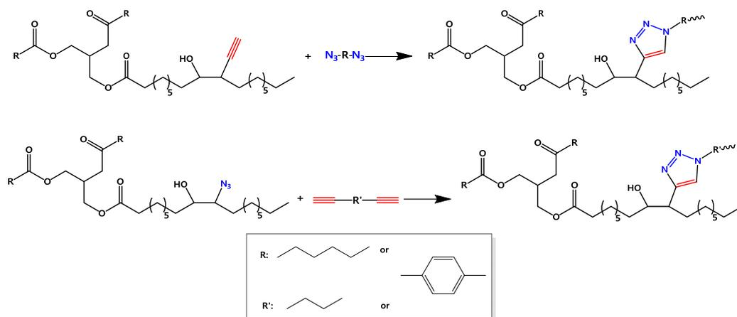
**Scheme 32.** CuAAC polymerization of azidated and alkynated soybean oils.
