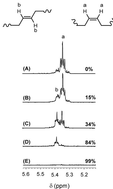
**Figure 1.** Expanded region (5.2-5.6 ppm) of the 400 MHz  $^1\text{H}$ -NMR spectra ( $\text{CDCl}_3$ ) during the photoinitiated thiol-ene click addition 3-mercaptopropionic acid to oleic acid as a function of conversion.
