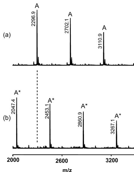
**Figure 4.** Expanded MALDI-TOF MS spectra of (a) alkenyl-terminated oligomer UDA-A3 ( $M_n^{\text{NMR}} = 2970$ ) and (b) the corresponding dihydroxy derivative UDA-OH3 obtained by photoinitiated thiol-ene click with ME.
