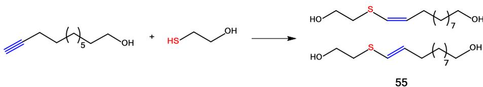
**Scheme 28.** Synthesis of a vinyl sulphide diol by thiol-yne addition of ME to UDYO.
