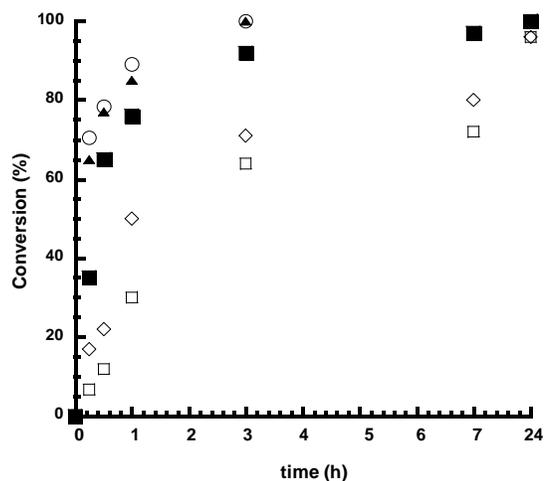
**Figure 7.** Nucleophilic substitution of PE-Br (M<sub>n</sub>=9KDa) with different nucleophiles in 1.2: 1 NuH: Br molar ratio: 2-mercaptoethanol (M<sub>n</sub>: 9KDa)(○), 2-mercaptoethanol (M<sub>n</sub>: 30KDa)(▲), 2-aminoethanol (□), propionic acid (■) and poly(N-isopropylacrylamide)(◊).
