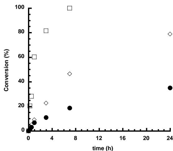
**Figure 4.** Nucleophilic substitution of DMBS with carboxylic acids in different COOH/Br molar ratio: glycolic acid (1:1) and 1 mol KF/1 mol COOH (●), glycolic acid (1.2:1) and 2 mol KF/1 mol COOH (◇), propionic acid (1.2:1) and 2 mol KF/1 mol COOH (□).
