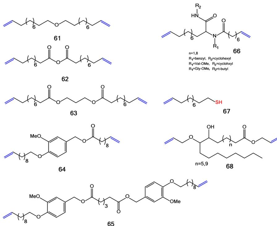
**Scheme 34.** Synthesis of  $\alpha,\omega$ -diene monomers based on fatty acids for thiol-ene polymerization.
