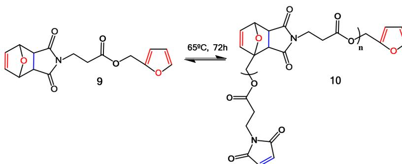
**Scheme 6.** DA polymerization of a furan-maleimide monomer.
