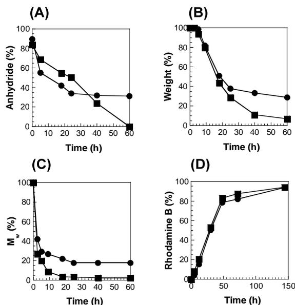
**Figure 3.** Evolution of % anhydride bonds (A), % weight (B), %  $M_w$  (C) during the hydrolytic degradation of PA-UDS (■) and PA-UDS:UDTGS (80:20) (●) conducted at 37 °C in phosphate buffer solution (pH 7.4). (D) Rhodamine B release studies carried out with polymer devices of PA-UDS and PA UDS-UDTGS (80:20) containing 5% of hydrophobic dye in phosphate buffer (pH=7.4) at 37°C.
