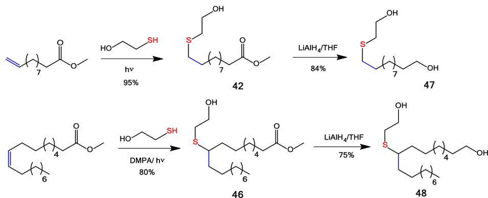
**Scheme 20.** Synthesis of diols via thiol-ene addition to undecylenic and oleic acid derivatives and subsequent reduction.
