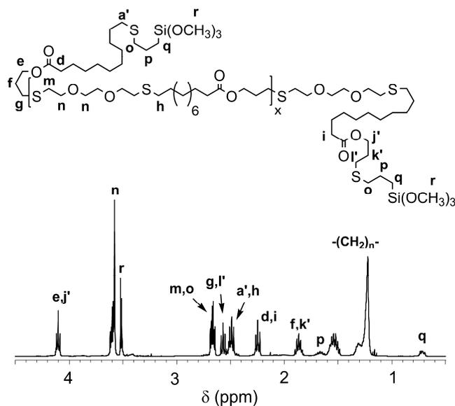
**Figure 7.** 400 MHz  $^1\text{H-NMR}$  spectra ( $\text{CDCl}_3$ ) of UDA-based telechelic with trimethoxysilane end groups (UDA-Si).
