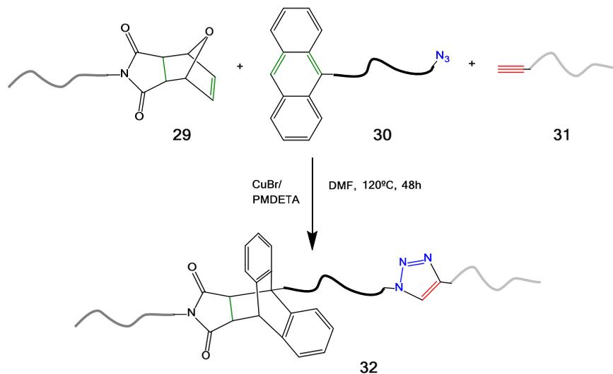
**Scheme 13.** Orthogonal one-pot synthesis of ABC triblock copolymers by simultaneous DA and CuAAC.
