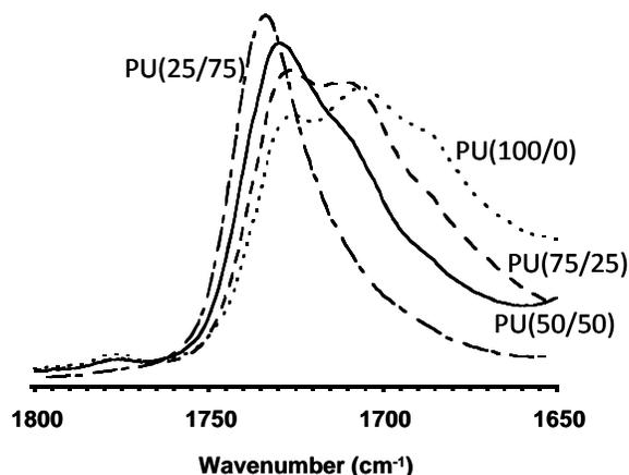
**Figure 3.** A section of FTIR spectra of PL(MUDY/UDYO)-derived PUs.
