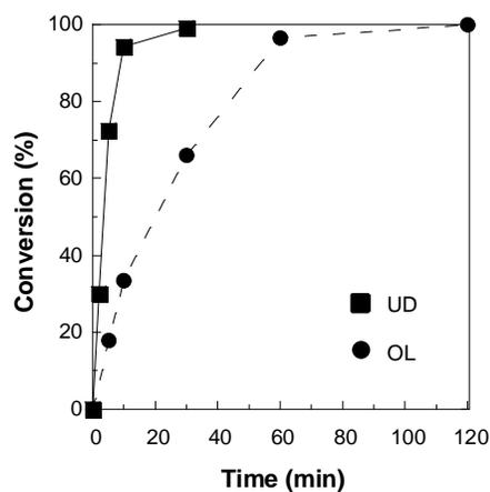
**Supporting Figure SF1.** Kinetic plots for the photoinitiated thiol-ene click coupling between 3-mercaptopropionic acid and (■)10-undecenoic acid and (●) oleic acid.
