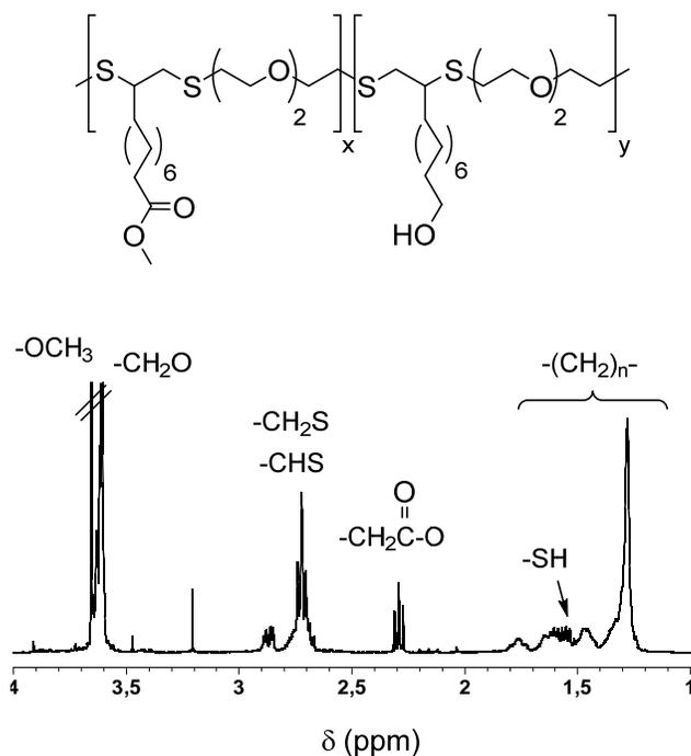
**Figure 2.** <sup>1</sup>H NMR spectrum of polyol PL(50/50)
