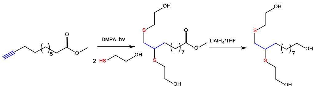
**Scheme 27.** Synthesis of a novel diol and triol via thiol-yne addition of ME to MUDY and subsequent ester-groups reduction.
