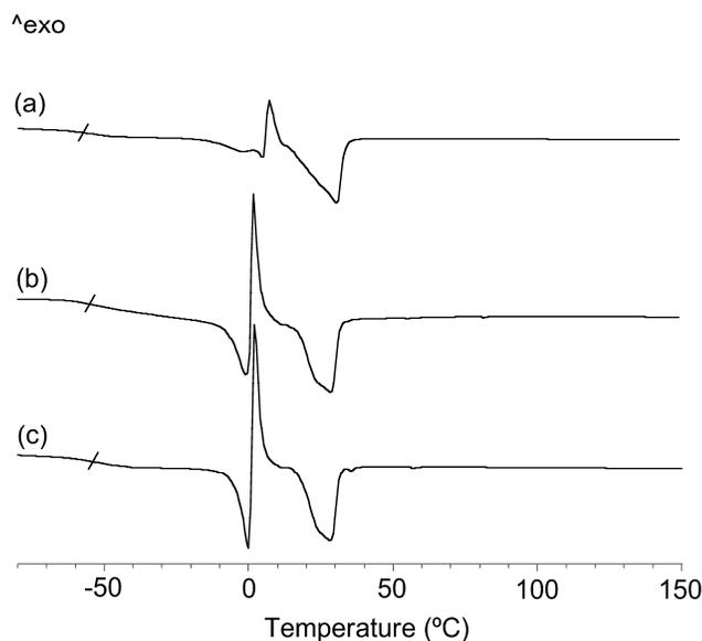
**Figure 6.** Second scan DSC traces (20°C/min) of UDA-based telechelic diols obtained by two consecutive thiol-ene couplings: (a) UDA-OH1 ( $M_n^{\text{NMR}} = 960$ ), (b) UDA-OH2 ( $M_n^{\text{NMR}} = 2060$ ), and (c) UDA-OH3 ( $M_n^{\text{NMR}} = 3100$ ).
