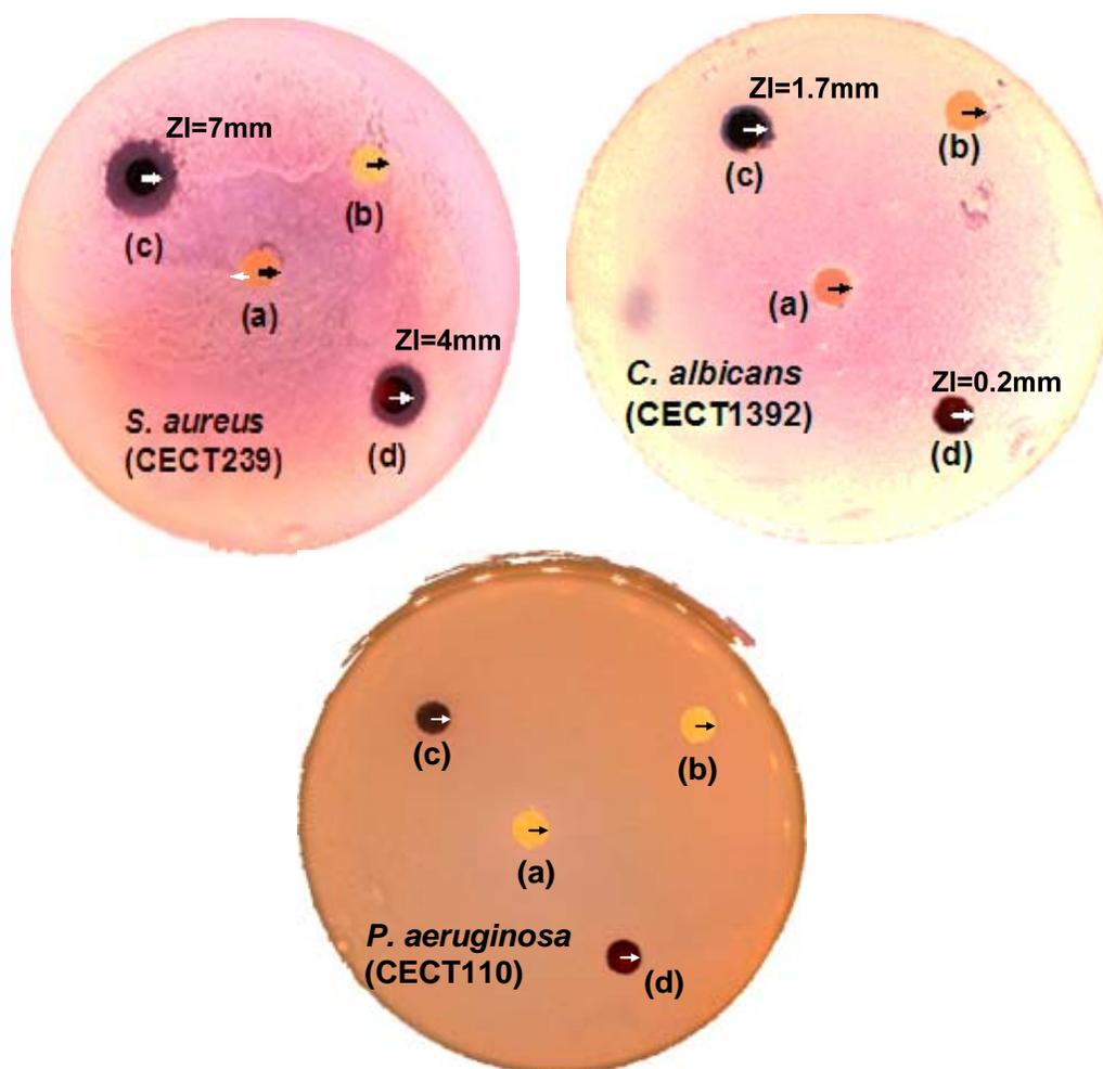
**Figure 7.** Antimicrobial test results for *S. aureus*, *C. albicans* and *P. aeruginosa* after 24h incubation. (a) PU(25/75) control, (b) PU(25/75) after 3h aminolysis treatment with Jeffamine/Propanol solution and PU(25/75) after aminolysis and iodine treatments containing (c) 2.8 wt-% I<sub>2</sub> and (d) 2 wt-% I<sub>2</sub>.
