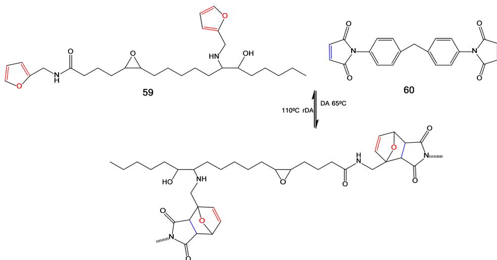
**Scheme 33.** DA polymerization of furan-functionalized linseed oil triglycerides.
