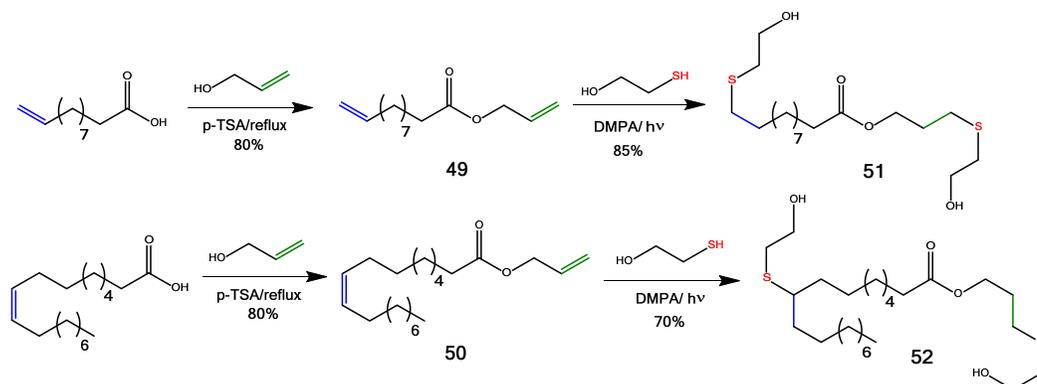
**Scheme 21.** Synthesis of diols via double thiol-ene addition to undecylenic and oleic acids.
