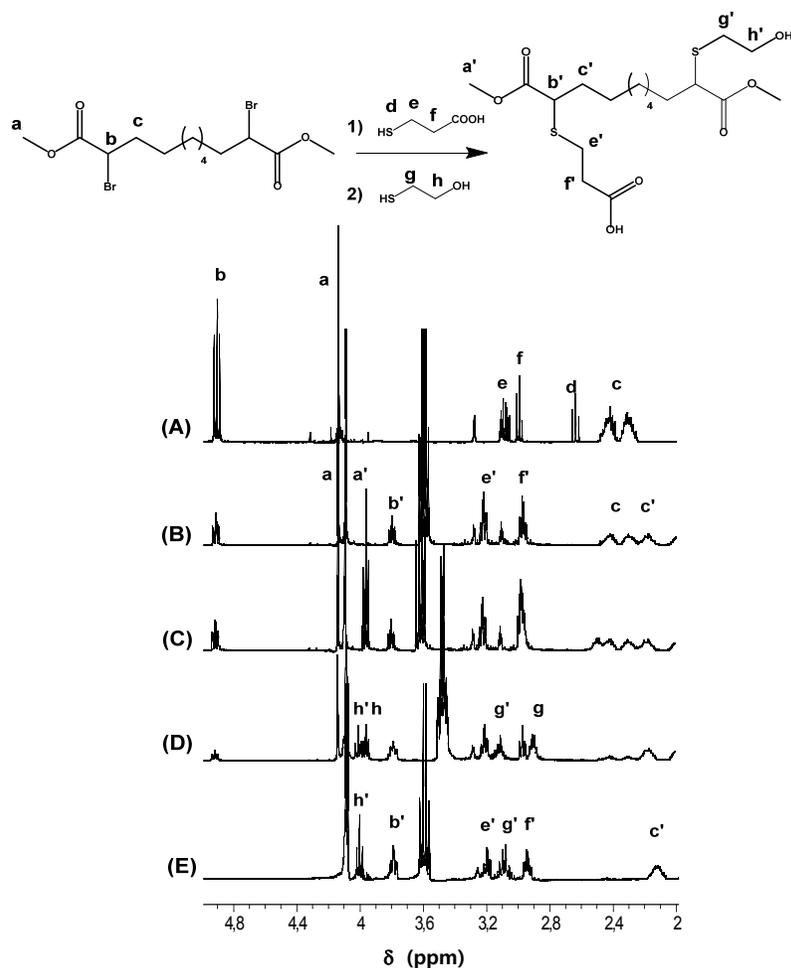
**Figure 2.**  $^1\text{H}$  NMR spectra of sequential nucleophilic substitution of DMBS with **2** and **1**: (A) DMBS and **2** at  $t=0$ ; (B)  $t=24\text{h}$ ; (C) Addition of **1**; (D)  $t=40\text{h}$ ; (E) Reaction product after 48h.
