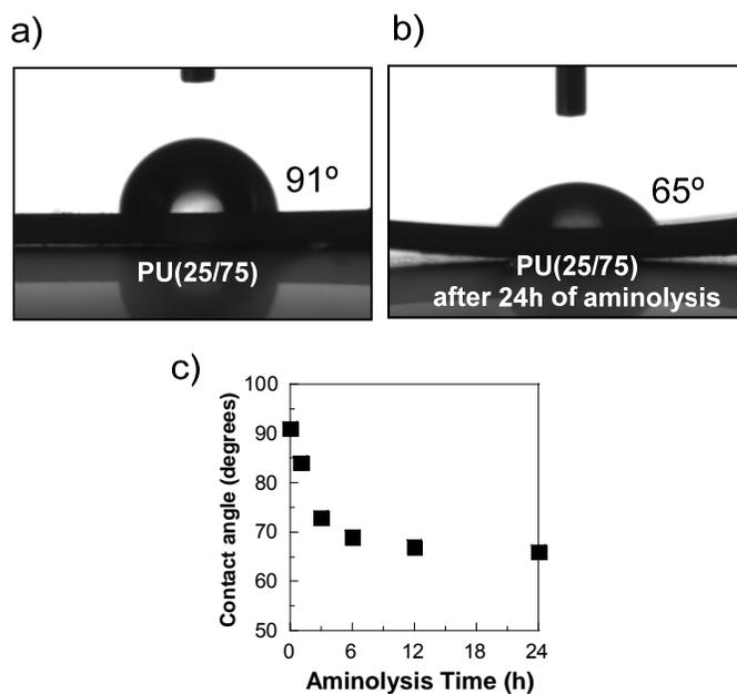
**Figure 4.** Contact angle images for PU(25/75) (a) before and (b) after 24h aminolysis treatment with Jeffamine/*i*Propanol solution. (c) Contact angle evolution with aminolysis time treatment for PU(25/75).
