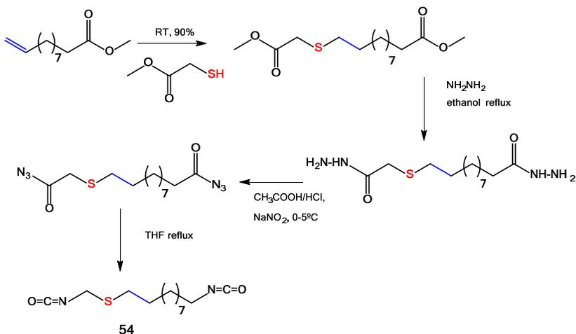
**Scheme 23.** Synthesis of a diisocyanate via thiol-ene chemistry.
