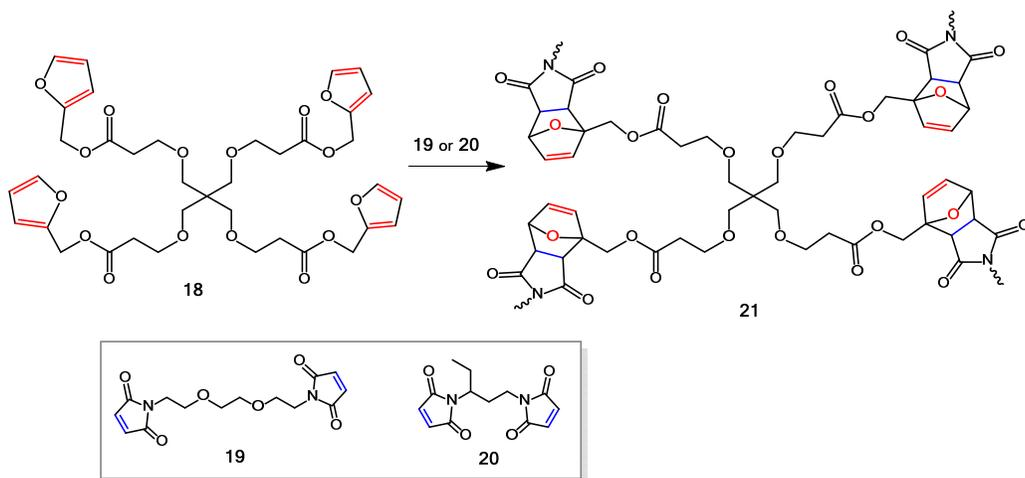
**Scheme 10.** Formation of self-reparable networks using reversible DA reactions.
