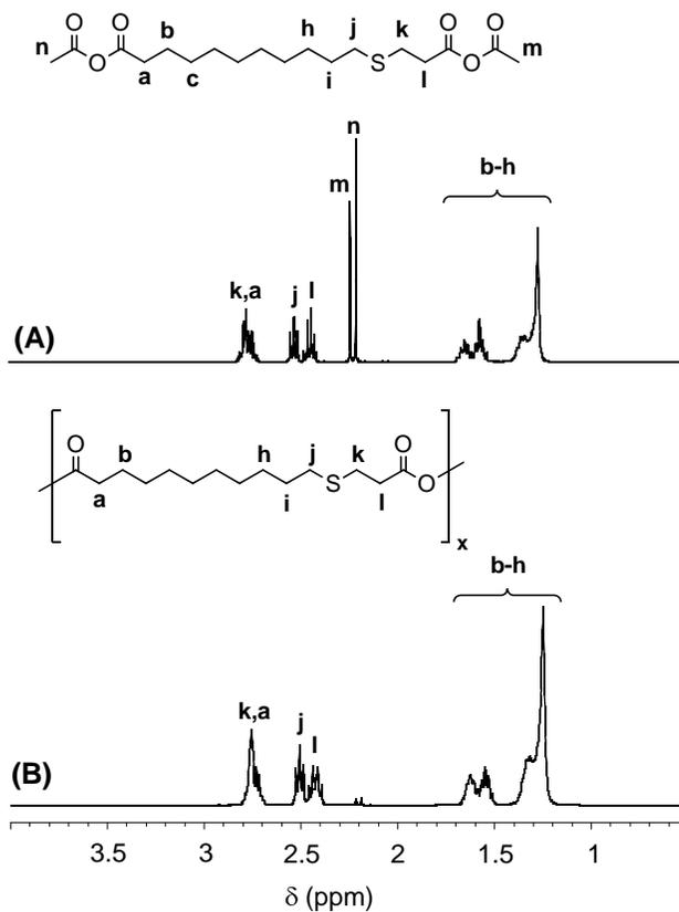
**Supporting Figure SF2.** 400 MHz <sup>1</sup>H-NMR spectra (CDCl<sub>3</sub>) of (a) acetylated UDS and (b) PA-UDS.
