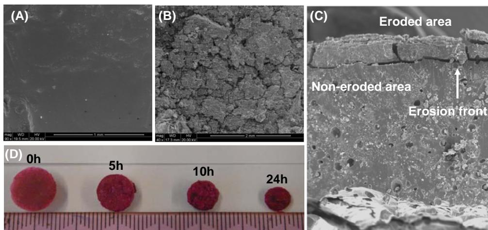
**Figure 4.** SEM micrographs of the outer surface and cross section of PA-UDS discs before and after degradation for 16 h in a phosphate buffer solution (pH 7.4) at 37°C. (A) Outer surface before degradation; (B) outer surface after degradation for 16 h; (C) cross section after degradation for 16h.
