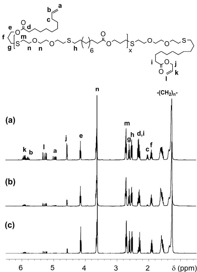
**Figure 1.** 400 MHz  $^1\text{H}$ -NMR spectra ( $\text{CDCl}_3$ ) of alkenyl-terminated UDA oligomers obtained by photoinitiated thiol-ene click step-growth polymerization with dithiol DT: (a) UDA-A1 (UDA/DT = 1.712;  $M_n^{\text{NMR}} = 895$ ), (b) UDA-A2 (UDA/DT = 1.259;  $M_n^{\text{NMR}} = 2060$ ), and (c) UDA-A3 (UDA/DT = 1.158;  $M_n^{\text{NMR}} = 2970$ ).
