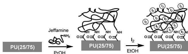
**Scheme 2.** Schematic illustration for the two steps surface modification of PU(75/25) with Jeffamine M-600 and iodine.
