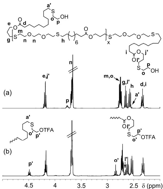
**Figure 5.** Expanded 400 MHz <sup>1</sup>H-NMR spectra (CDCl<sub>3</sub>) of (a) telechelic diol UDA-OH<sub>2</sub> and (b) the corresponding bistrifluoroacetylated derivative.
