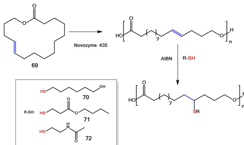
**Scheme 35.** Post-polymerization modification of the main chain.
