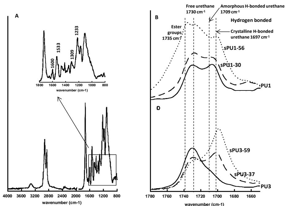
**Figure 1.** FTIR spectra of (A) PU3; (B) PU1 series; (C) PU3 series.
