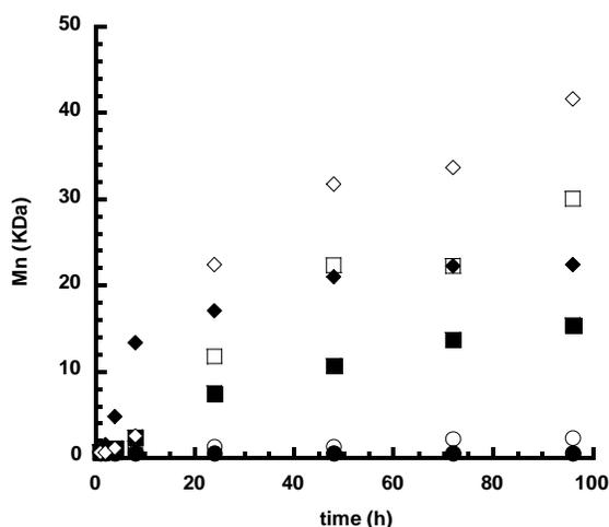
**Figure 5.** Mn vs. polymerization time for the polymerization of DMBS and DCD using different catalysts concentration (% w/w Novozyme/DMBS). Open symbols for solution polymerization and solid symbols for bulk polymerization. (○ 10%, □ 20%, ◇ 40%).
