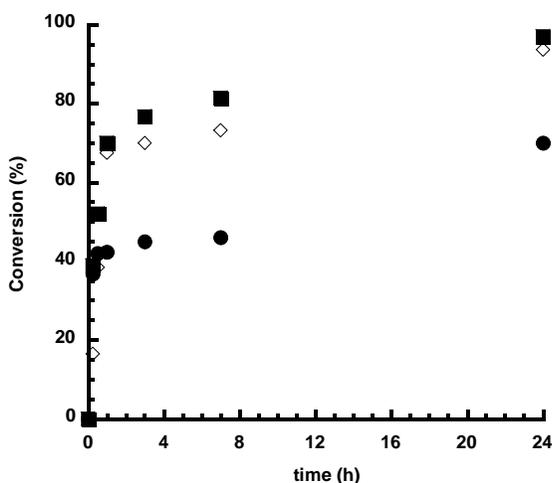
**Figure 3.** Nucleophilic substitution of DMBS with amines in different  $\text{NH}_2/\text{Br}$  molar ratio: 2-aminoethanol (1:1) (●), 2-aminoethanol (1.1:1) and 2 mol  $\text{NEt}_3$ /1 mol  $\text{NH}_2$  (◇), 2-aminoethanol (1.2:1) and 2 mol  $\text{NEt}_3$ /1 mol  $\text{NH}_2$  (■).
