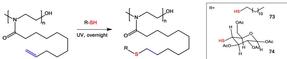
**Scheme 36.** Post-polymerization modification of the side chains of alkene-functionalized poly(oxazoline)s.
