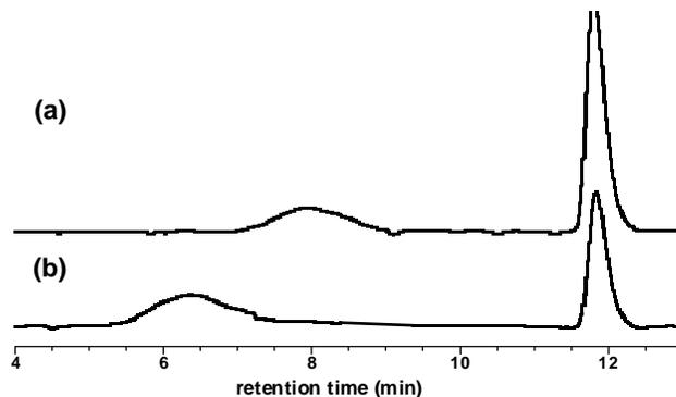
**Figure 8.** SEC measurements of: a) PE-Br and b) PE-Br modified with NIPAAm-COOH.
