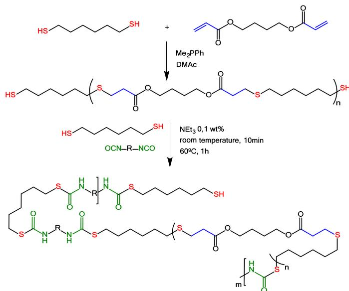
**Scheme 7.** Synthetic procedure for segmented polythiourethane elastomers.
