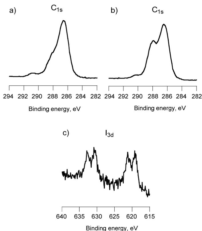
**Figure 6.** C<sub>1s</sub> spectra for (a) PU(25/75) control and (b) after 3h aminolysis treatment with Jeffamine/*i*Propanol solution. (c) I<sub>3d</sub> spectrum of PU(25/75) after aminolysis and iodine treatments.
