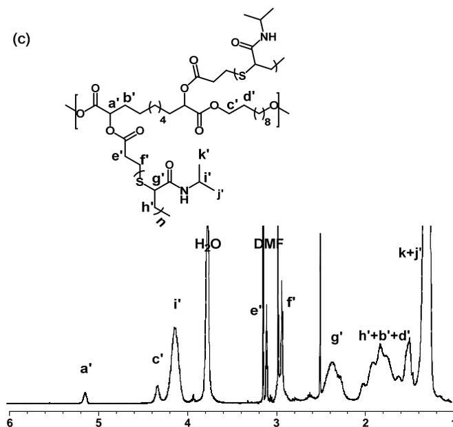
**Figure 6.** <sup>1</sup>H NMR spectra of a) PE-Br polyester (M<sub>n</sub>=9KDa); b) PE-Br modified with propionic acid; (c) PE-Br modified with NIPAAm-COOH.
