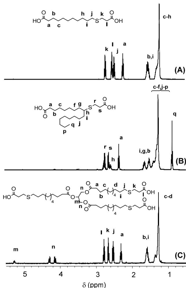
**Figure 2.** 400 MHz <sup>1</sup>H-NMR spectra (CDCl<sub>3</sub>) of biobased carboxylic acids synthesized via thiol-ene addition: (A) UDS, (b) OLS, and (C) UDTGS.
