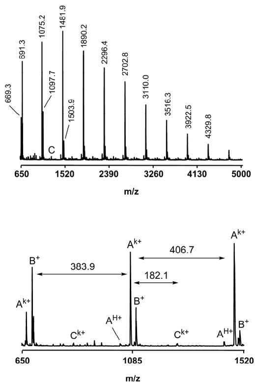
**Figure 2.** MALDI-TOF MS spectrum of alkenyl-terminated oligomer UDA-A3 ( $M_n^{\text{NMR}} = 2970$ ) obtained by photoinitiated thiol-ene click step-growth polymerization with dithiol DT (UDA/DT = 1.158).
