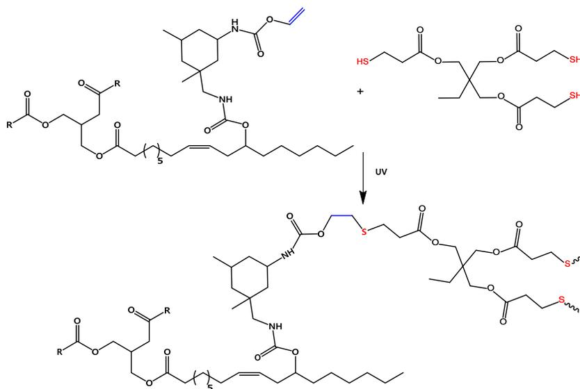
**Scheme 30.** Thiol-ene photopolymerization of vinyl ether-based castor oil.
