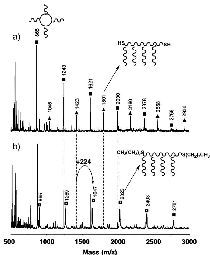
**Figure 1.** MALDI-TOF spectra of PL(MUDY/DT) (a) before and (b) after thiol-ene reaction with an excess of 1-octene in the presence of DMPA as a photoinitiator under UV light.
