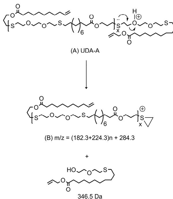
**Scheme 2.** Suggested Fragmentation Pathway of Alkenyl-terminated UDA Oligomers during MALDI-TOF Analysis.
