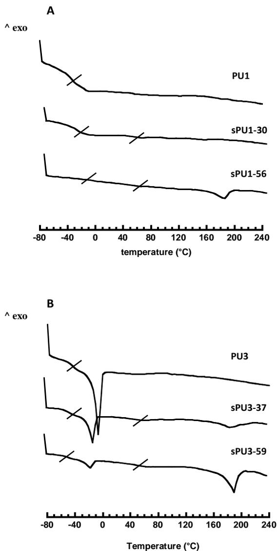
**Figure 2.** DSC thermograms of (A) PU1 series; (B) PU3 series.
