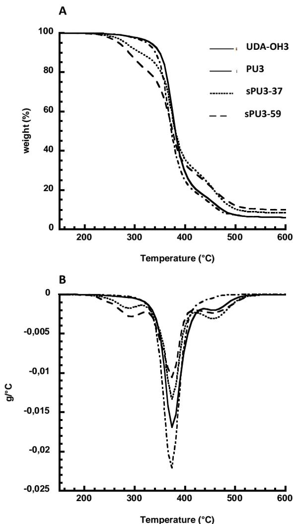
**Figure 3.** TGA traces of sPU3 series: (A) weight loss curves; (B) first derivative curves.
