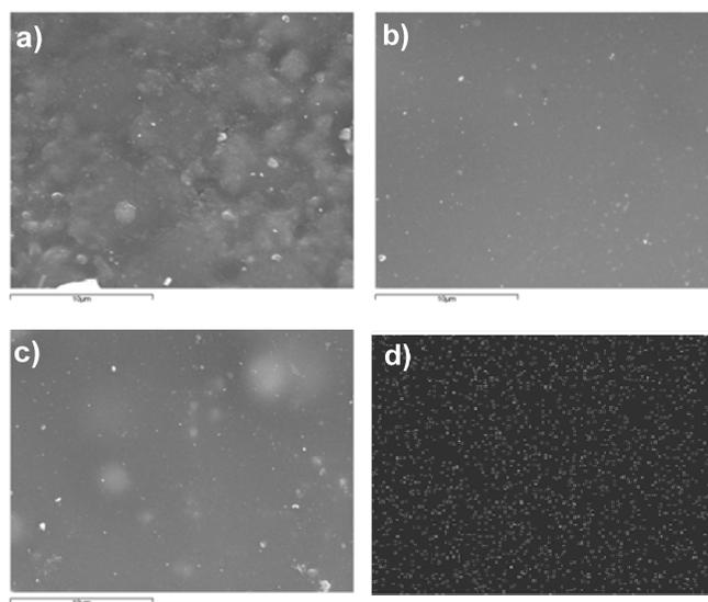
**Figure 5.** SEM micrographs of (a) PU(25/75) control, (b) after 3h aminolysis treatment with Jeffamine/iPropanol solution, and (c) after 3h immersion in a iodine/ethanol solution. Micrograph (d) corresponds to iodine Ka X-ray map of the PU(25/75) after aminolysis and iodine treatments.
