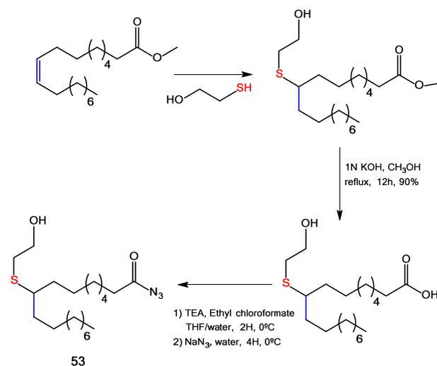
**Scheme 22.** Synthesis of an hydroxy-acyl azide monomer derived from methyl oleate using thiol-ene chemistry.
