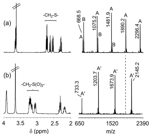
**Figure 3.** Expanded 400 MHz <sup>1</sup>H-NMR (CDCl<sub>3</sub>) and MALDI-TOF MS spectra of alkenyl-terminated UDA oligomer UDA-A3 (a) before and (b) after oxidation with 3-chloroperbenzoic acid.
