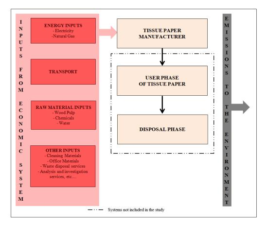
Figure 4.1: EIO-LCA system description of tissue paper production
