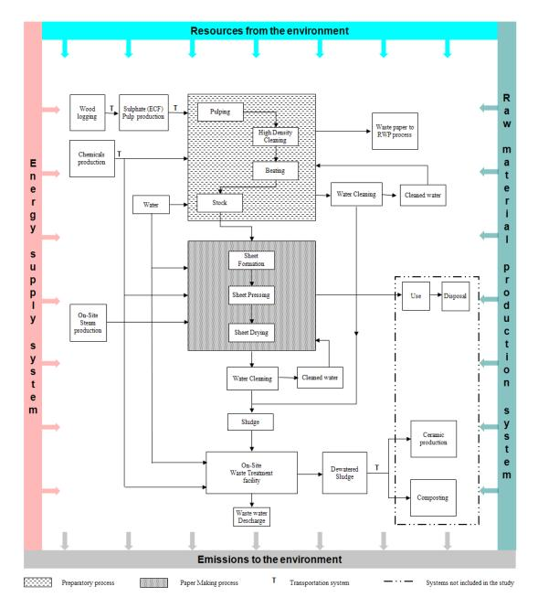
Figure 3.1: LCA system boundary and process flows of tissue paper production from  $\mathrm{VP}$
