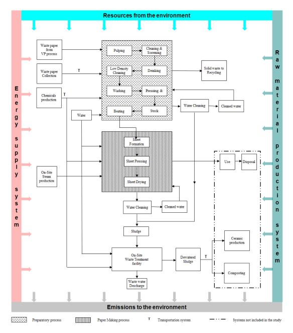
Figure 3.2: LCA system boundary and process flows of tissue paper production from RWP  $\,$
