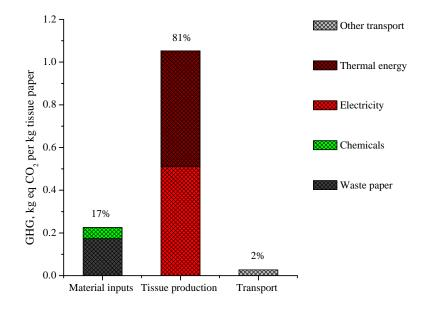
Figure 3.4: Contribution to GHG emissions of inputs during tissue paper production using RWP process
