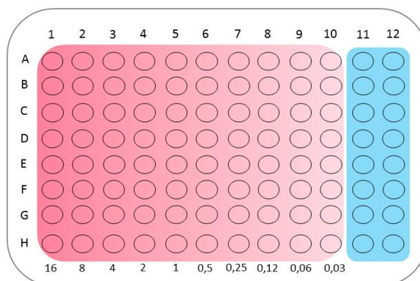
**Figure 6. Schematic distribution of the different antifungal concentrations in a range of 0.03 to 16  $\mu\text{g}/\text{ml}$ . Columns 11 and 12 are used as negative (-) and positive (+) controls, respectively.**
