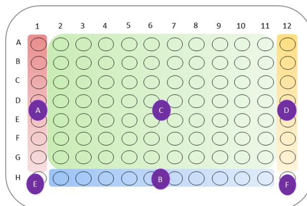
**Figure 7. Representation of the distribution of antifungal compounds in a 96-well microplate testing a double combination. Six zones are defined: A and B, zones to determine the minimal inhibitory concentration (MIC) of each antifungal alone; C, zone of antifungal combination; D, defined as the zone of positive control without antifungal; E and F, defined as the zone of negative controls.**
