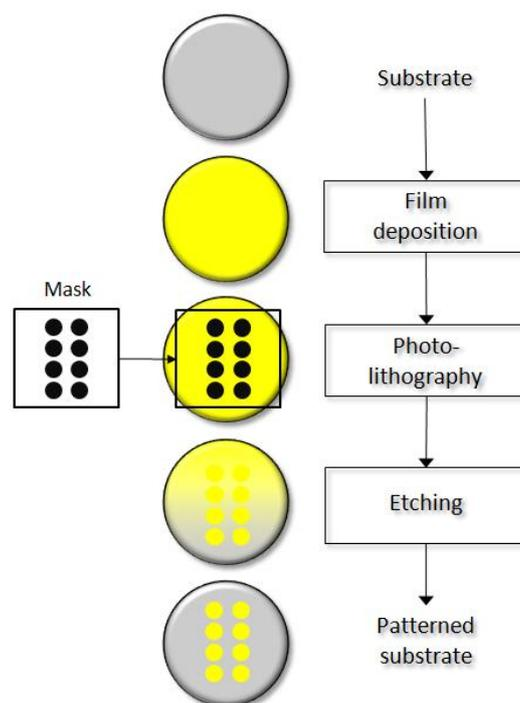
**Figure 1.10.** Flow diagram of an integrated circuit (IC)-based fabrication process using the three basic microfabrication techniques: film deposition, photolithography and etching.
