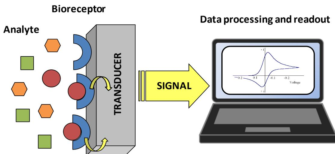
Figure 1.3. Main components in a biosensor
