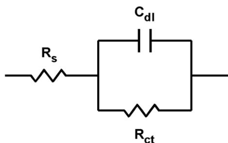
Scheme 2.2. Equivalent circuit used to model the impedance data ( $R_s$ : solution resistance,  $R_{ct}$ : resistance to charge transfer,  $C_{dl}$ : double layer capacitance).
