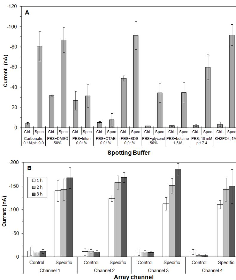
**Figure 5.3.** Electrochemical response of both specific (Spec.) and control (Ctrl.) electrodes for (A) various spotting buffers for the PCB microarray functionalisation using the LabNext XactII arrayer (10 nM solution of URP was used as target); and (B) three immobilization times (1, 2 and 3 hours) of the thiolated CD24 capture probe (5 nM solution of complementary CD24 was used as target). Each bar corresponds to the average current of 8 electrodes.
