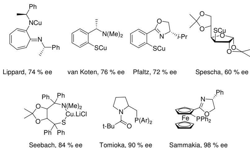
**Figure 33.** Heterocuprate-based ligand and chiral ligands using Grignard reagents.
