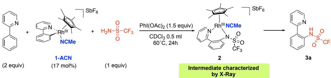
**Scheme 12.** Catalytic reaction where crystals were observed to be formed. Stoichiometric reactions gave the same coordinated product.
