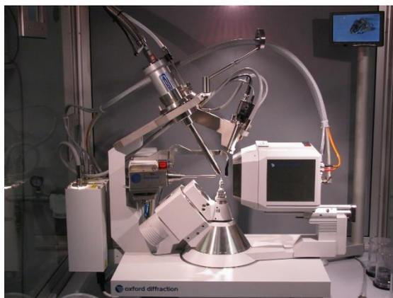
**Figure 9.** Single crystal X-ray diffractometer. A crystal is mounted and displayed in the screen placed at the top right. Image has been taken from the literature.<sup>19</sup>
