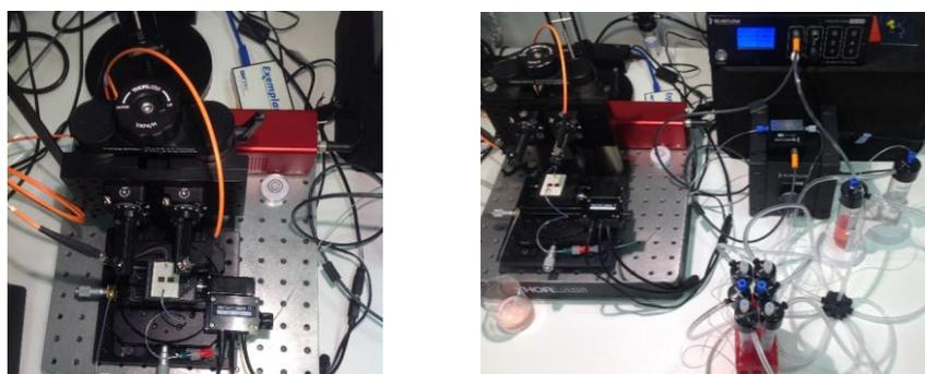
*Figure 6. Nanostructured plasmon biosensor based on Blu-ray disc connected to a microfluidic system prepared for the biodetection.*
