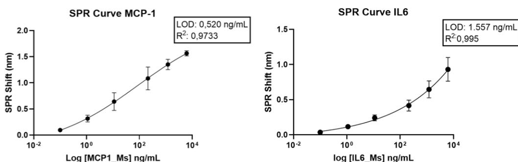
Figure 20. SPR biosensor calibration curve. Left, MCP-1 SPR calibration curve. Right, IL-6 SPR calibration curve
