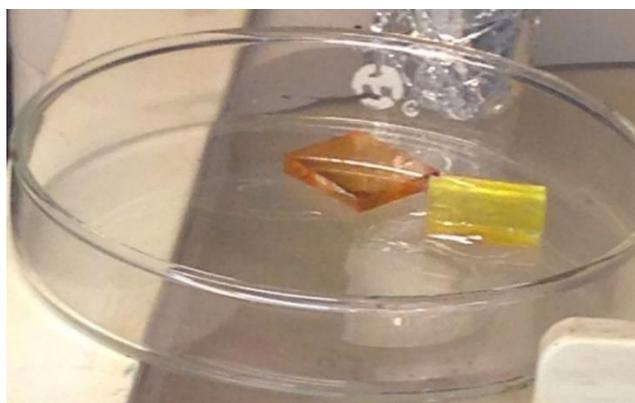
**Figure 17:** *the spin-coating of the perovskites into the films lasted 30 seconds. When the second film was spin-coated, the first one was already orange.*
