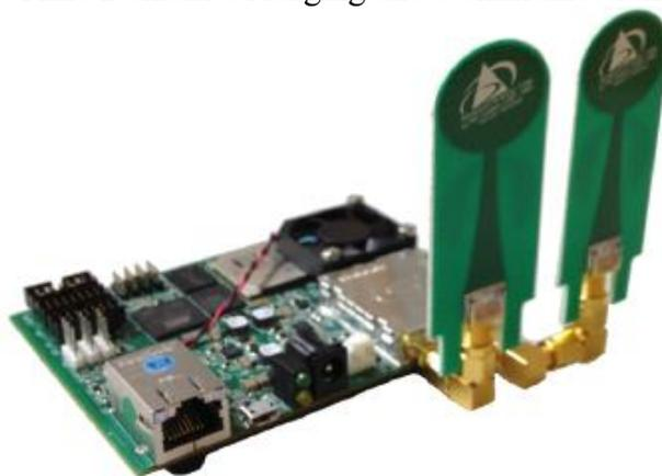
Fig. 7.1 P400 MRM with pair of attached Broadspec antennas
