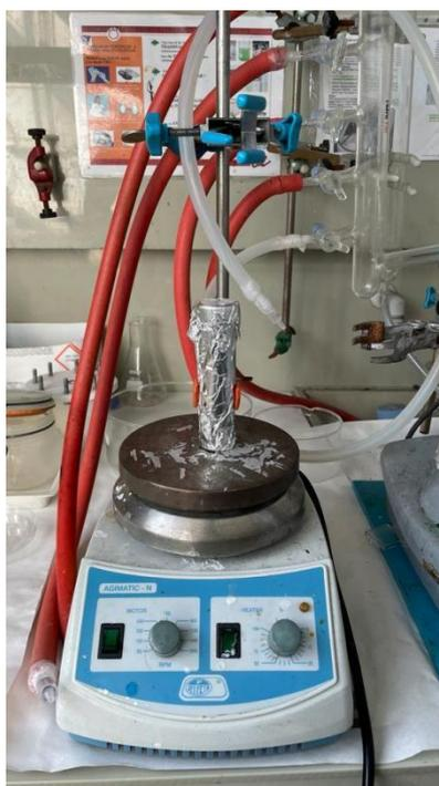
**Figure 26.** Mounting of the NAA samples dipped in 1 mg/ml of DOX solution on the stirrer overnight.
