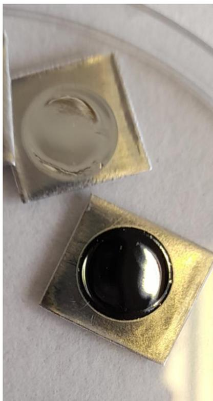
**Figure 9.** Electropolished aluminium foils.
