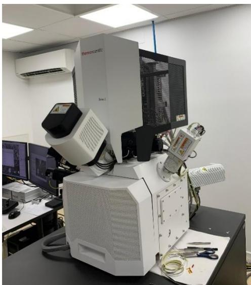
**Figure 15.** FESEM microscopy equipment
