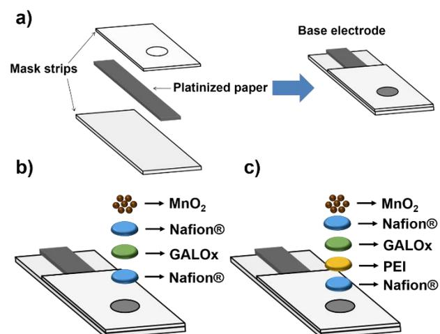
**Figure 2.** a) Scheme of the construction of the base-electrode and methods for GALOx immobilization, b) sandwiching and c) crosslinking.
