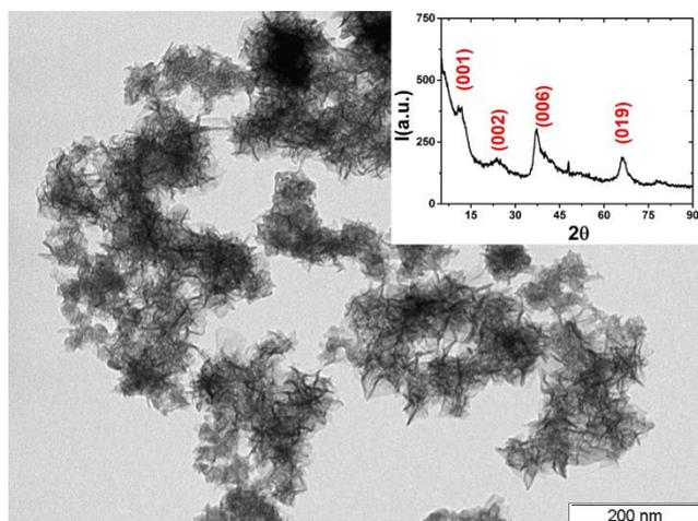
**Figure 3.** TEM image of MnO<sub>2</sub> nanoparticles. Inset: DRX pattern. The (*hkl*) planes are indicated.
