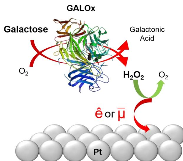
**Figure 1.** Scheme of electrochemical strategies for measurements of galactose.
