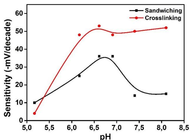
**Figure 6.** Influence of working pH on the sensitivity of the galactose sensors.
