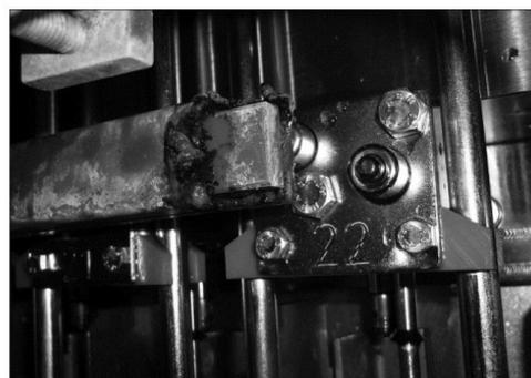
Fig. 6. Biofilm on a release ledge of filling valves in the filler release area – the site is beyond the reach of central foaming system.
