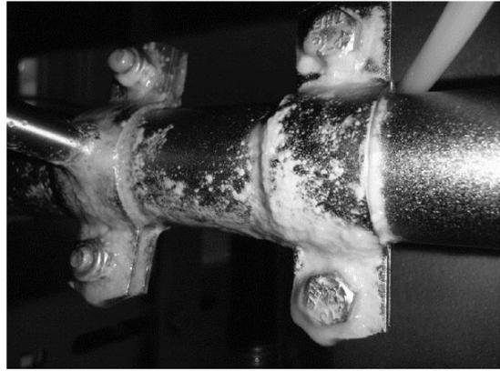
Fig. 3. Biofilm on construction elements in the monoblock and conveyor belt sampling area.
