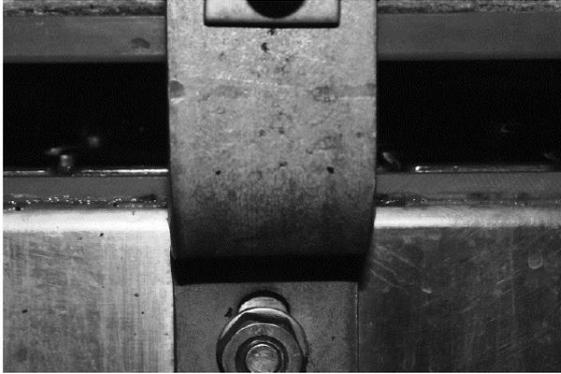
Fig. 1. Biofilm on the side ledge of the conveyor belt cover.
