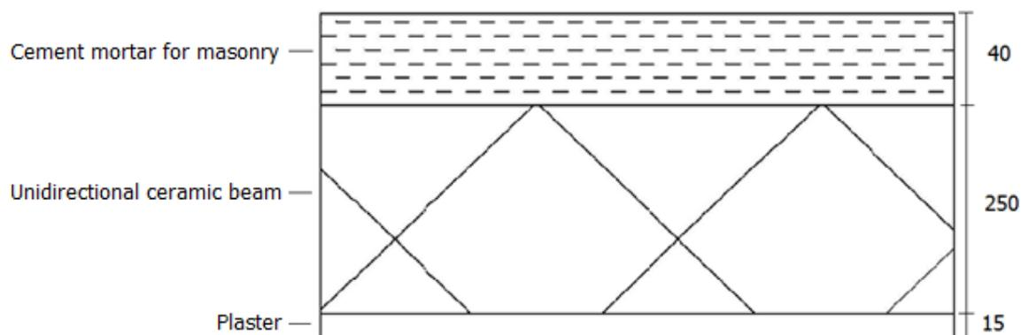
Figure 10. Interior ceiling elements diagram.
