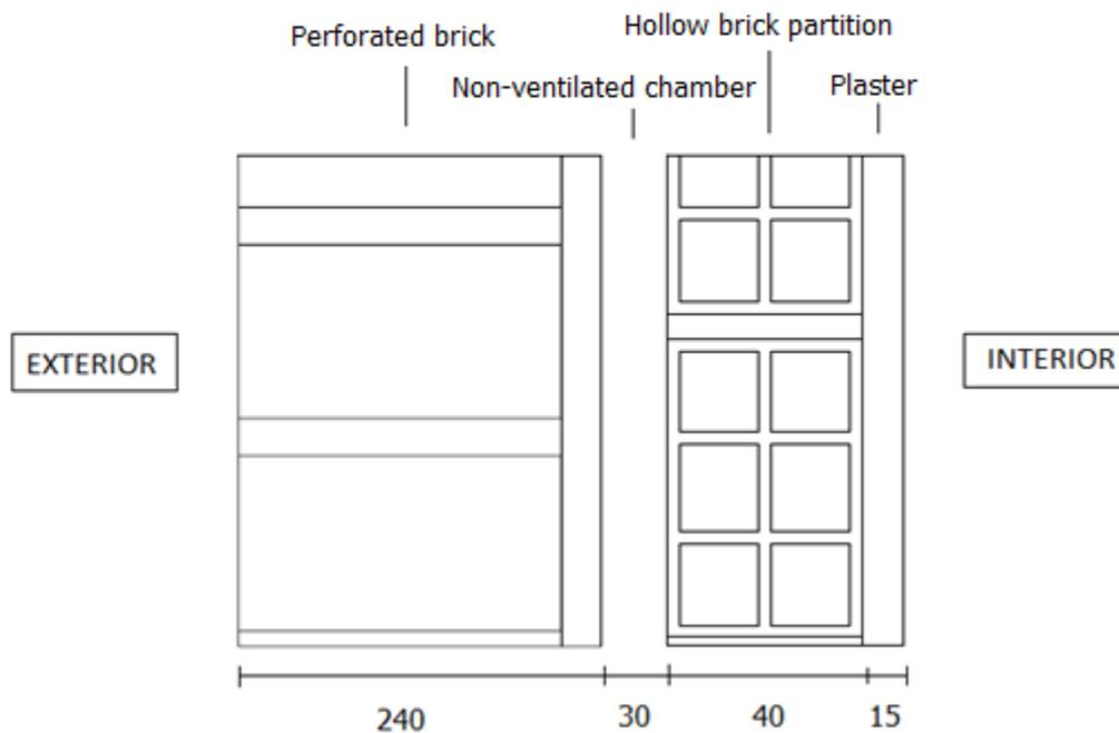
Figure 7. Exterior wall elements diagram [35].
