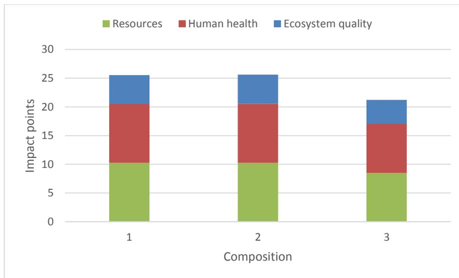
Figure 16. Effect of earth composition in the environmental impact points.
