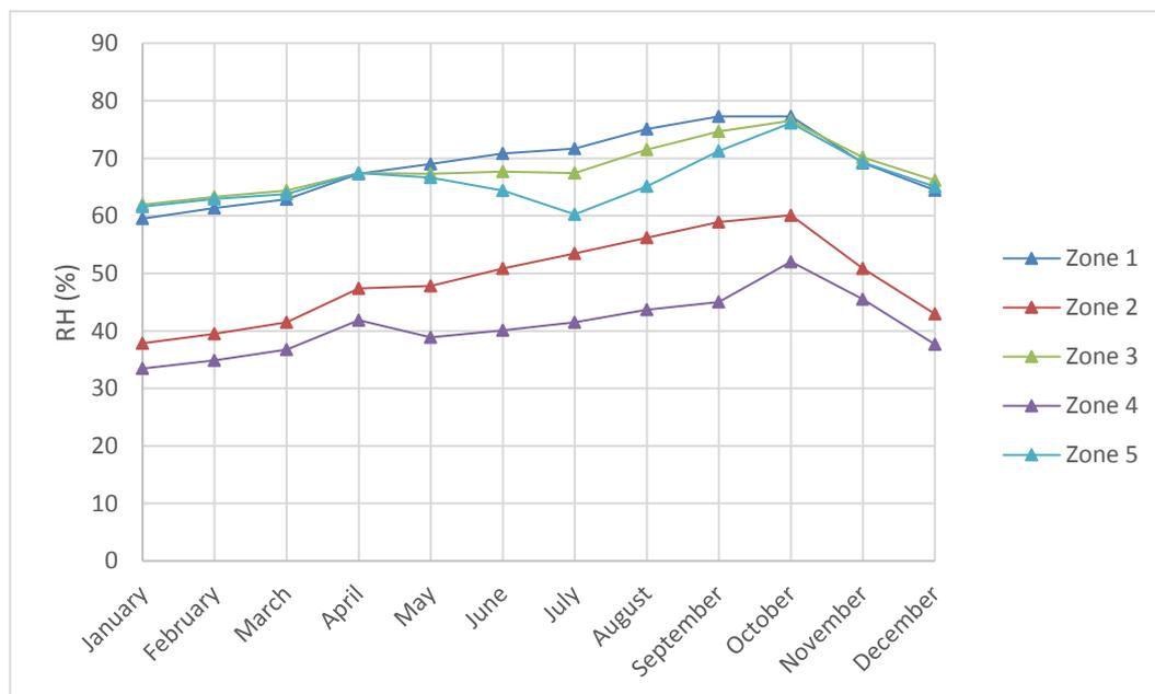
Figure 22. Silty clay loam case relative humidity results
