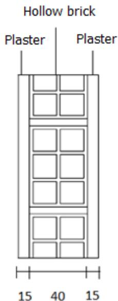
Figure 8. Interior wall elements diagram [35].
