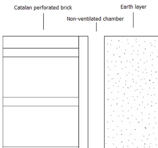
Figure 14. Exterior wall structure with earth.
