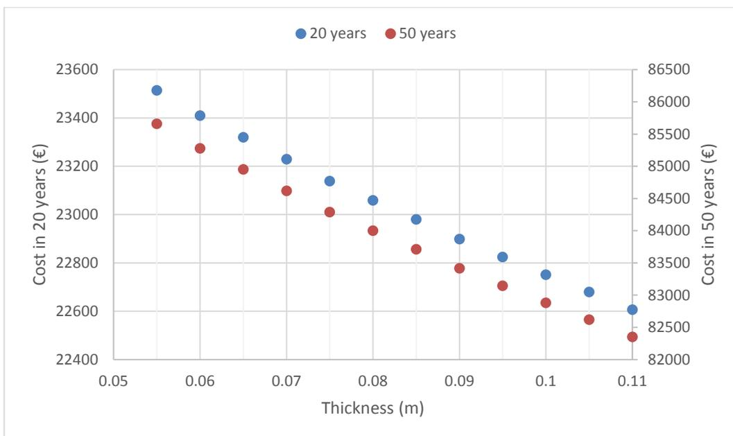
Figure 19. Parametric study cost evaluation in 20 and 50 years.
