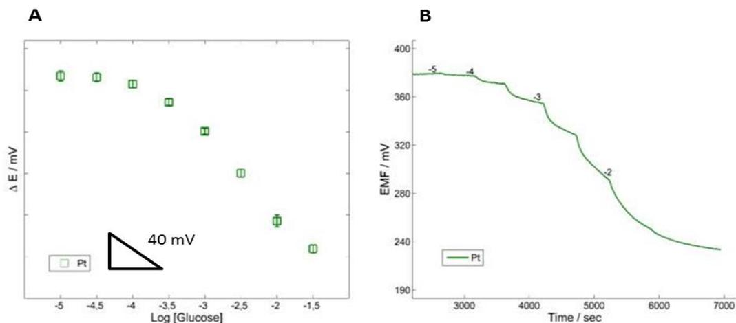
**Figure 5.** Potentiometric response of paper-based electrodes with detection of glucose: (A) calibration and (B) corresponding time-trace curves of paper-based reference electrode and platinum working electrode (in a 4 mL cell).
