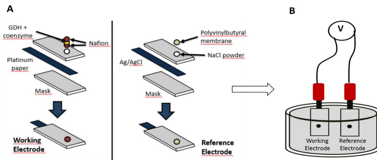
**Figure 1.** (A) Scheme for the construction of the working and reference electrodes. Working electrode: a layer of Nafion; a layer of GDH enzyme with NAD coenzyme; a layer of Nafion. Reference electrode: layer of NaCl and reference membrane. (B) Picture containing sensors in the cells connected with potentiometer.
