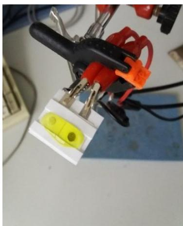
**Picture 1.** Picture showing the new "channel" design, connected with potentiometer and detection of glucose.
