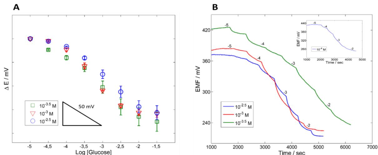
**Figure 4.** Comparison of the sensitivity and reproducibility of platinum electrodes with optimization of different concentration of PMS mediator, (A) calibration curve and (B) time-trace.
