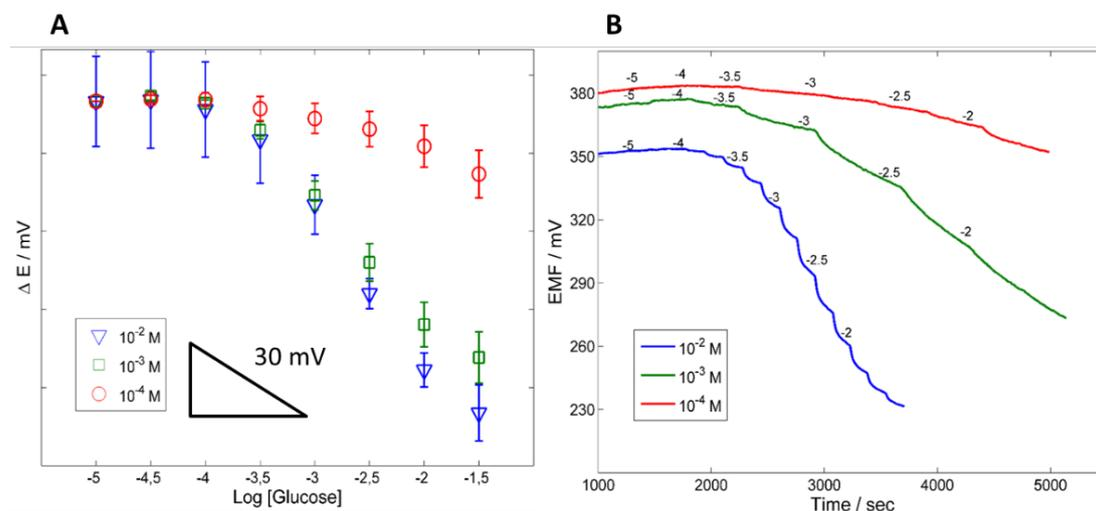
**Figure 3.** Comparison of the sensitivity and reproducibility of platinum electrodes with optimization of different concentration of NAD coenzyme, (A) calibration curve and (B) time-trace.
