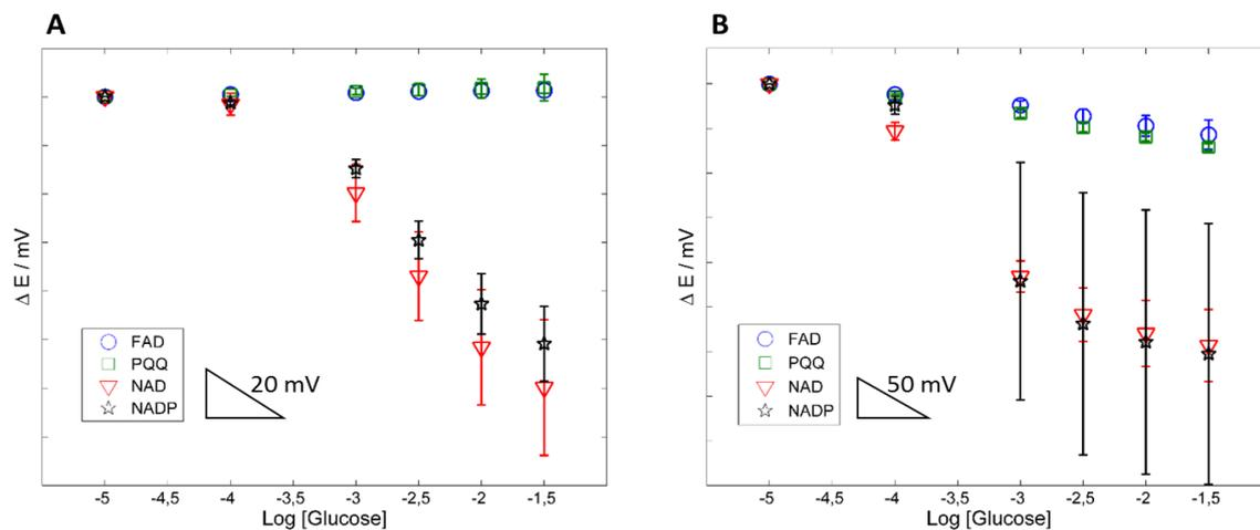
**Figure 2.** Calibration curve of optimization of coenzymes with increasing concentration of glucose for (A) platinum electrodes and (B) gold electrodes.
