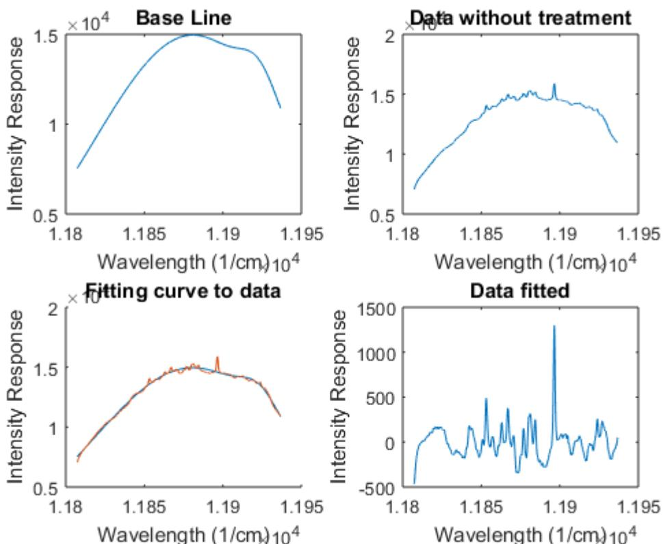
Figure 1: Model of fitting curve in Raman spectra.
