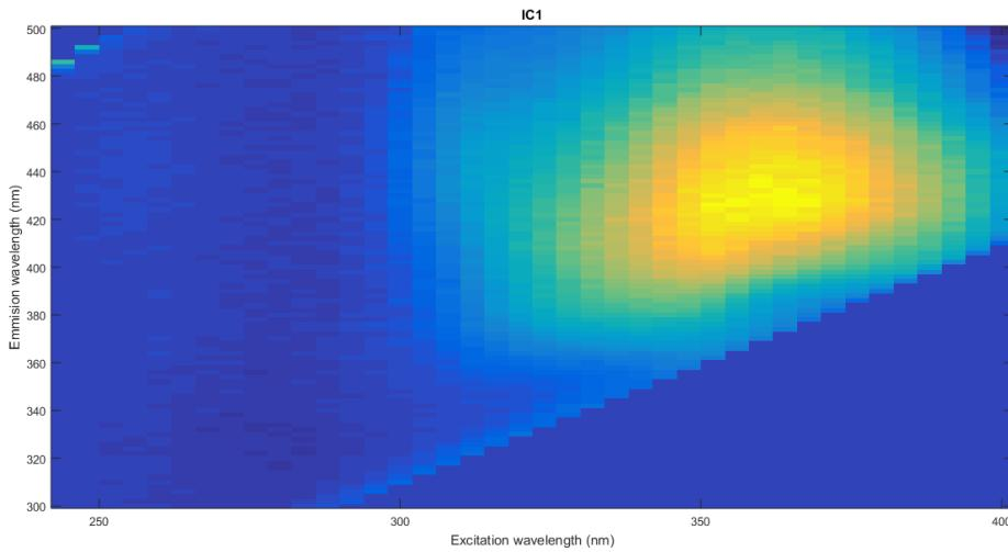
**Figure 5:** Signal extraction of ICA (IC1) at day 1 in 3D-FFFS (Excitation wavelength (245-400 nm)-Emission wavelength (300-500 nm)).
