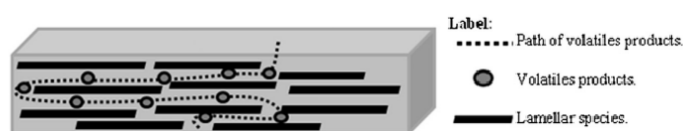
Figure 2. Schematic representation of physical barrier effect provided by the MMT in a polymeric matrix. Extracted from [19].
