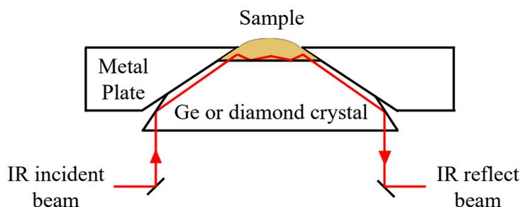
**Figure 1.** Description of the main parts of the ATR device.
