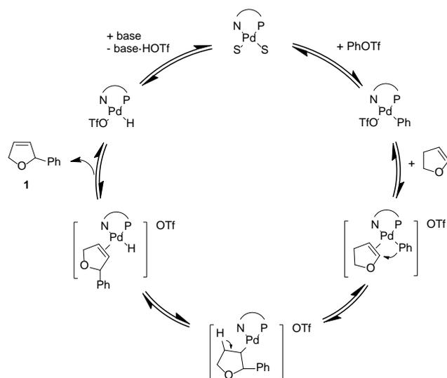
**Scheme 8.** Accepted mechanism for the asymmetric Pd-catalyzed Heck reaction of **S1**.
