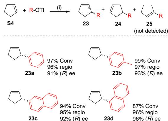
**Scheme 6.** Asymmetric Heck reaction of cyclopentene **S4**. (i) 2.5 mol% [Pd<sub>2</sub>(dba)<sub>3</sub>] $\cdot$ C<sub>6</sub>H<sub>6</sub>, 5.6 mol% **L2d**, <sup>i</sup>Pr<sub>2</sub>NEt (2 equiv), THF, 50 °C, 48 h.
