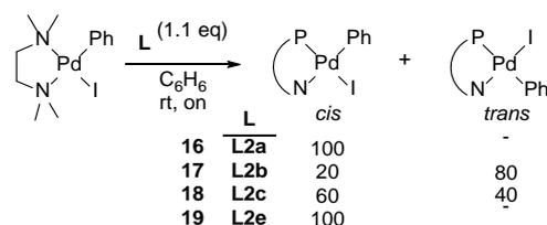
**Scheme 3.** Preparation of [Pd(I)(Ph)(L)] (**L=L2a-c,e**) neutral complexes. The ratio of each isomer measured by <sup>31</sup>P-NMR spectroscopy is also shown.
