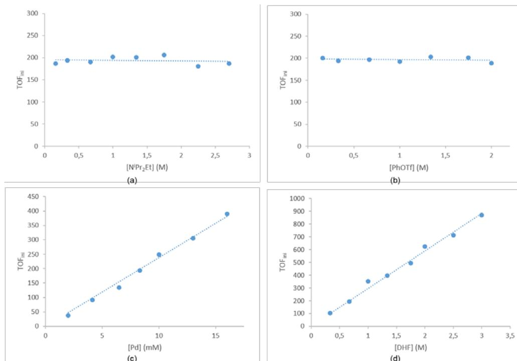
**Figure 3.** Kinetic measurements. Plots of  $\text{TOF}_{\text{ini}}$  versus (a)  $[\text{N}^i\text{Pr}_2\text{Et}]$ , (b)  $[\text{PhOTf}]$ , (c)  $[\text{Pd}]$  and (d) **S1** for the reaction of **S1** with PhOTf in THF at 50 °C catalyzed by complex  $[\text{Pd}(\text{Ph})(\text{OTf})(\text{L2a})]$ .  $\text{TOF}_{\text{ini}}$  measured after 1 h (conversions typically of 5-10%).
