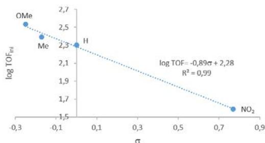
**Figure 4.** Hammett plot showing the effect of substituents on the Heck reaction using catalytic system Pd/L2a.
