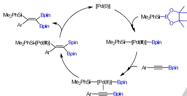
**Scheme 16.** Suggested mechanism for the palladium-catalyzed silaboration of alkynylboronates.
