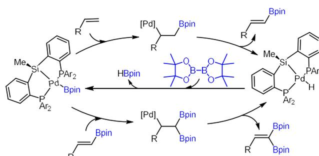
**Scheme 14.** Suggested mechanism for the palladium-catalyzed double dehydrogenative borylation of alkenes.
