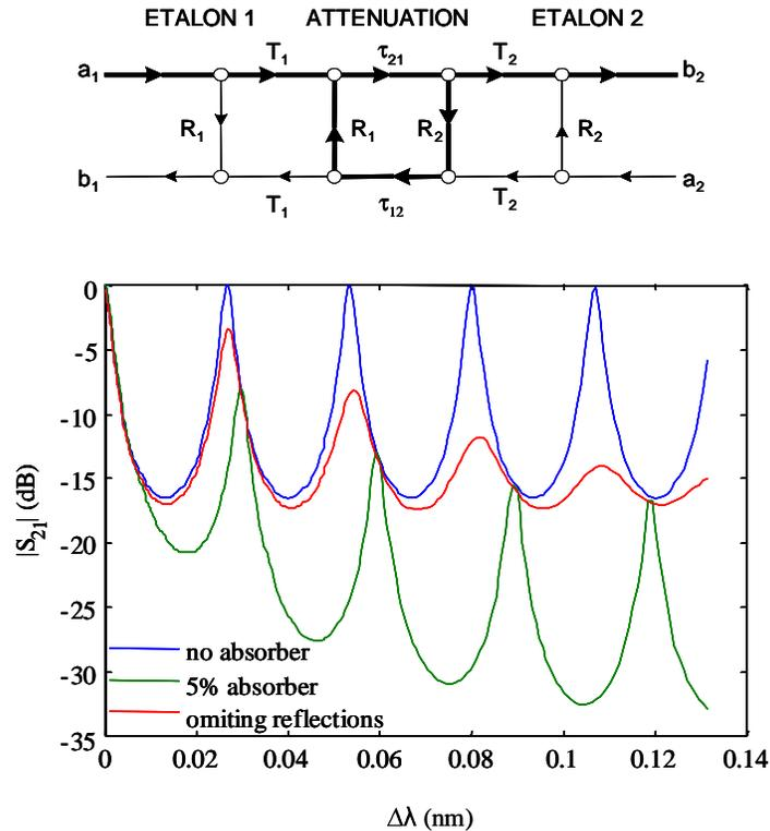
Fig. 4. Flow chart (up) for two etalons with a attenuator used to reduce reflections between etalons. In bold line, it is marked the signal path for an input wave that propagate to the output of the second etalon. Transmittance for the dual-etalon solar filter without absorber, with 5% absorber, and isolated etalons omitting reflections (down).
