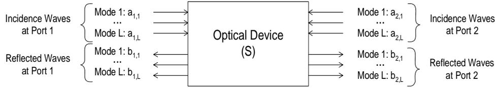
Fig. 1 Outgoing and incoming waves in two-port optical network. We denote the incoming and outgoing waves at ports  $i$  by the  $L=(2M+1) \times (N+1)$ -component vectors  $a_i$ , and  $b_i$ , respectively
