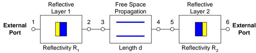
Fig. 2. A Fabry-Perot interferometer can be analyzed as a multiport optical system composed of three different two-port elements. Waves  $b_2$  transmitted by the first reflective layer propagated a distance  $d$  to reach the second reflective layer as incoming waves  $a_5$ . By properly defining the scattering matrix of any of these three elements, our modal approach allows to describes any interference and diffractive problem characterizing the Fabry-Perot etalon behavior.
