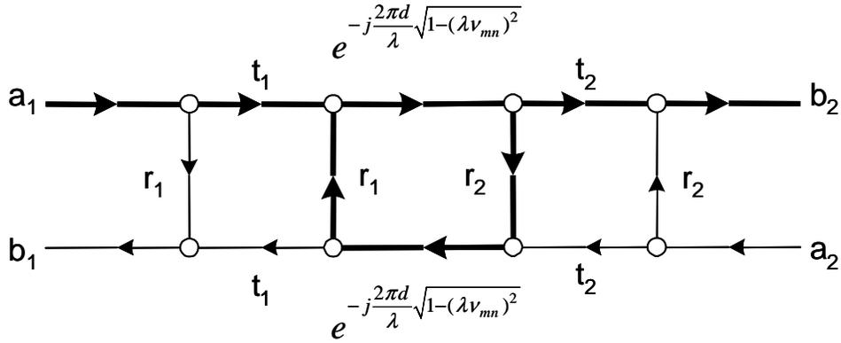
Fig. 3. Flow chart for a Fabry-Perot interferometer. In bold line, the signal path for an input wave that propagates to the output of the etalon. To find the transfer function of the etalon system represented by this block diagram we use Mason's gain rule.
