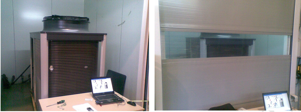
Figure 2. Air-cooled prototype in the climatic chamber testing facility
