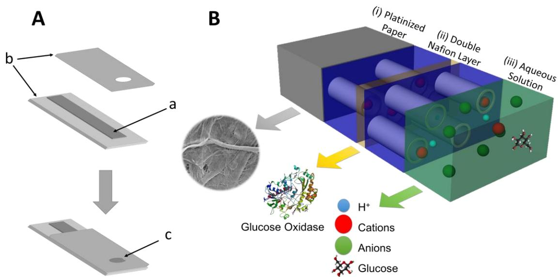
**Fig. 1.** Illustration of the paper-based biosensor. (A) Fabrication of the electrode, using a strip of platinized paper (a), sandwiched between two plastic masks (b), with a window of electroactive surface(c). (B) Scheme of the enzymatic membrane: (i) Pt-Paper Substrate; (ii) enzyme (GOx) sandwiched between two layers of Nafion, one at Pt-interface and the other at the (iii) solution interface.
