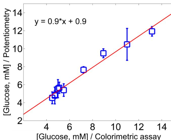
**Fig. 5.** Comparison of glucose determination (mM) in real samples obtained by the potentiometric paper-based electrode (mean±S.D., N=3) and colorimetric assay (data provided by the local hospital) at 25°C.
