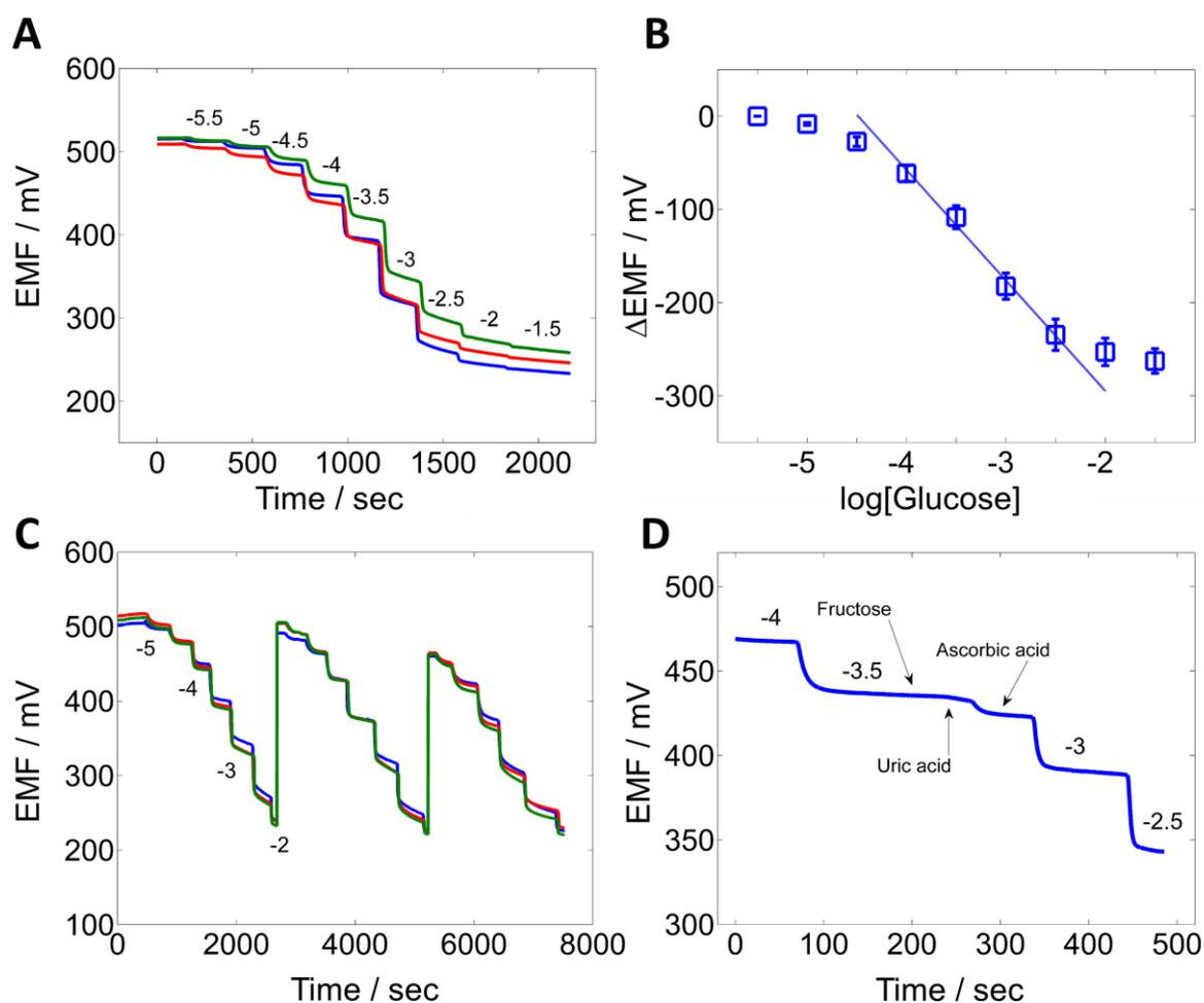
**Fig. 4.** Analytical performance of the paper-based enzymatic electrode: (A) Time-trace plot of three different electrodes in three separated potentiometric cells, (B) the corresponding calibration curve of enzymatic
