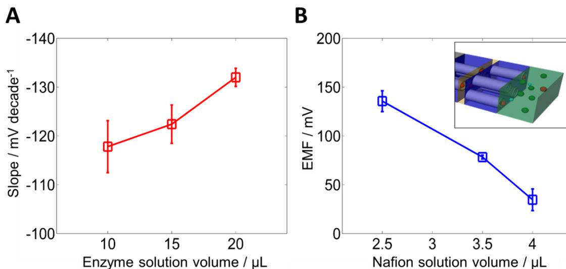
**Fig. 3.** Optimization of the analytical conditions for the biosensor. (A) Sensitivity for glucose vs volume of solution of enzyme concentration (20 mg/mL) cast. (B) Change on the potentiometric signal after the addition of  $10^{-4}$  M ascorbic acid as function of the increasing volume of Nafion membrane cast. In all cases, error bars correspond to the standard deviation of 3 different electrodes.
