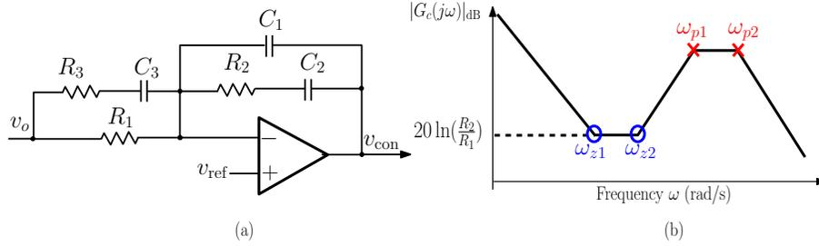
Figure 2. Schematic circuit diagram of a type-III compensator (a) and the modulus of its frequency response (b).
