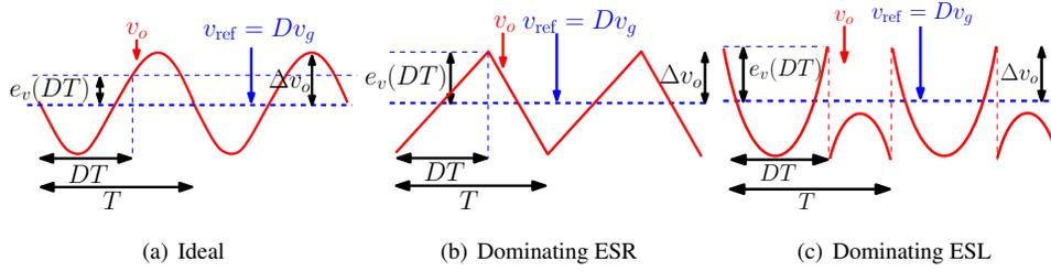
Figure 3. Waveforms of the output voltage ripple of a buck converter. (a) Ideal with null or very small ESR and ESL, (b) Dominating ripple due to ESR. (c) Dominating ripple due to ESL.
