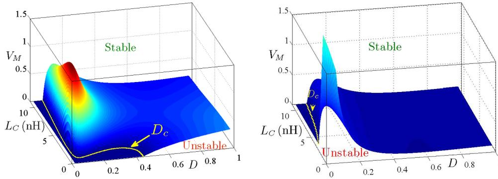
Figure 5. Stability boundary of the buck converter under  $V^1$  (a) and conventional type-III (b) compensation designs by showing the effect of the ESL  $L_C$  on the stability boundary.
