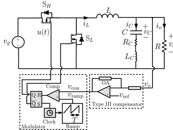
Figure 1. Schematic circuit diagram of a buck converter with the output capacitor modeled as an RLC network and under type-III compensation scheme.
